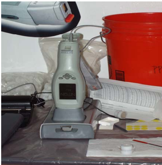
Figure 6-1. Niton XLi 700 Series analyzer set up for ex-situ analysis.
