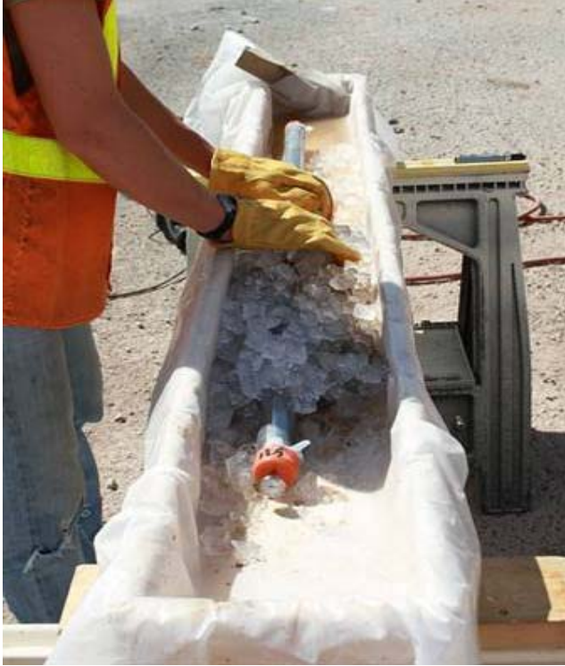
Figure 10. Hot soil core being cooled in ice bath, Grants, NM
