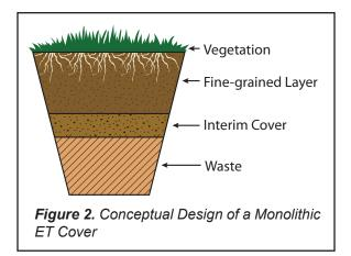
to as monofill covers, use a single fine-grained soil layer to retain water and support the vegetative community (Albright et al. 2010 and Hauser 2009). Figure 2 shows an example of a monolithic ET cover. Exhibit 1 provides an example of a full-scale monolithic cover at a MSW landfill.
