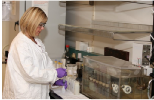
EPA researcher Karen Bradham uses a "virtual stomach" that mimics human digestion to determine if lead and arsenic in contaminated soils are bioavailable.
