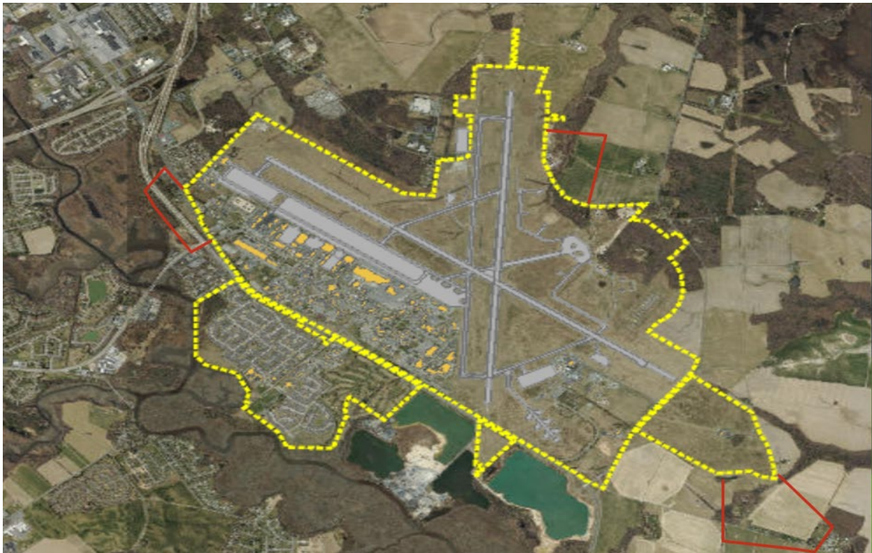
Figure 7: This aerial view shows off-base drinking water areas affected by PFAS at the Delaware Air Force Base site. Red polygons indicate known off-base contamination. The greatest distance to contamination is less than a half mile.
