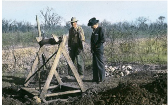
Barite (tuff) mining boomed in 1926 after the mineral's use for oil drilling mud was discovered. For a number of years, Washington County was the world's leading producer of barite. This 1937 photo shows a windlass used to raise tuff ore (photo credit: U.S. Forest Service [USFS]).
