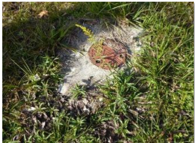
Figure 7. A groundwater monitoring well in the former school area.
