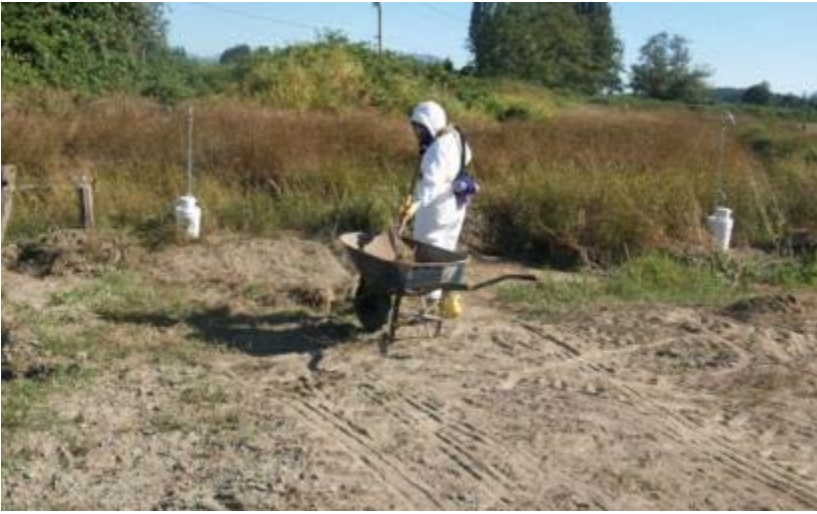
Digging soil scenario with perimeter monitorin
