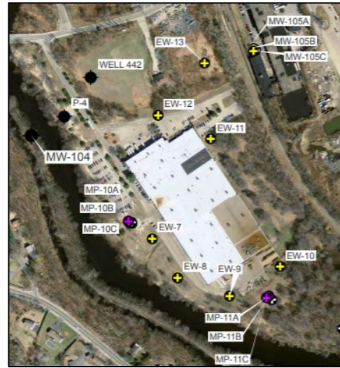
Monitoring recommendations for Peterson/Puritan Inc. OU01, from June 2016 Optimization Review. Appendix C Monitoring Optimization Results. Figure C.2
