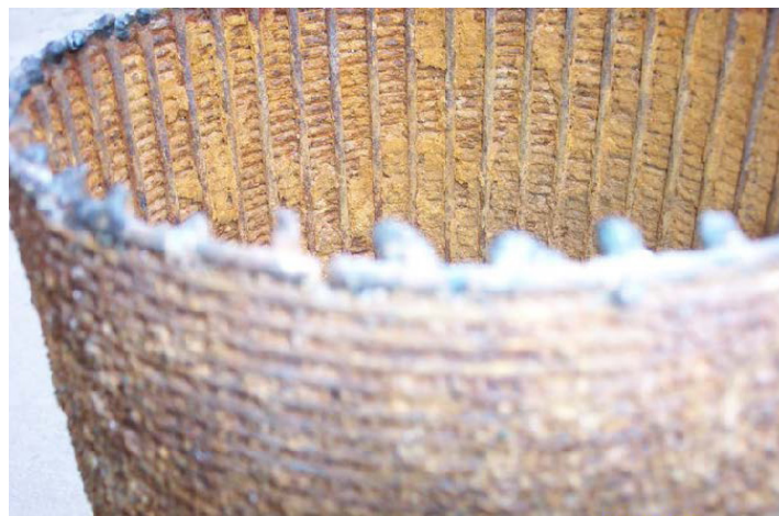
Figure 2. Well Screen Plugged with Metal Precipitates (Scherer, 2013).
