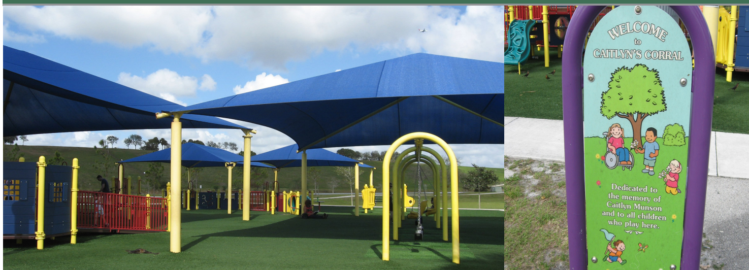
Caitlyn's Corral, one of the park's playgrounds. The universal-access playground is designed for special-needs children, and includes smooth surfaces, ramps, accessible swings and sound-play components.
