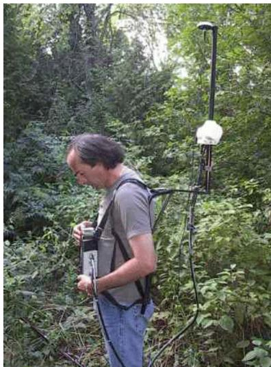
**Figure 6-12. GSM-19 Overhauser Proton Magnetometer with Gradiometer.**
