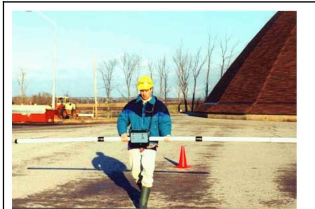
**Figure 6-8. Geonics EM-31 Terrain Conductivity Meter.**
