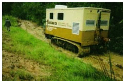
**Figure 5-2. All Terrain Cone Penetrometer Testing Rigs.**
