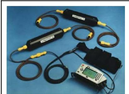
**Figure 6-4. Ohmmapper Resistivity Instrument.**
