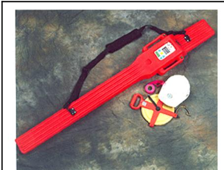
**Figure 6-7. GEM-300 Multi-frequency Terrain Conductivity Meter.**
