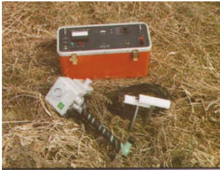
**Figure 6-9. EM16/EM16r VLF Receiver and TX 27 Transmitter.**
