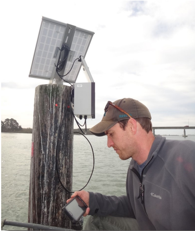
Water-quality monitoring station provides real-time data to interested parties, including oyster growers.
