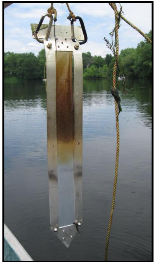
Figure 4-5. Photograph of LDPE in an aluminum frame after deployment in a freshwater lake sediment. The lower portion of the LDPE, which still appears transparent, was embedded below the sediment-water interface; in contrast, the LDPE in the lake bottom water was coated in material that may affect target contaminant uptake rates in the LDPE.
