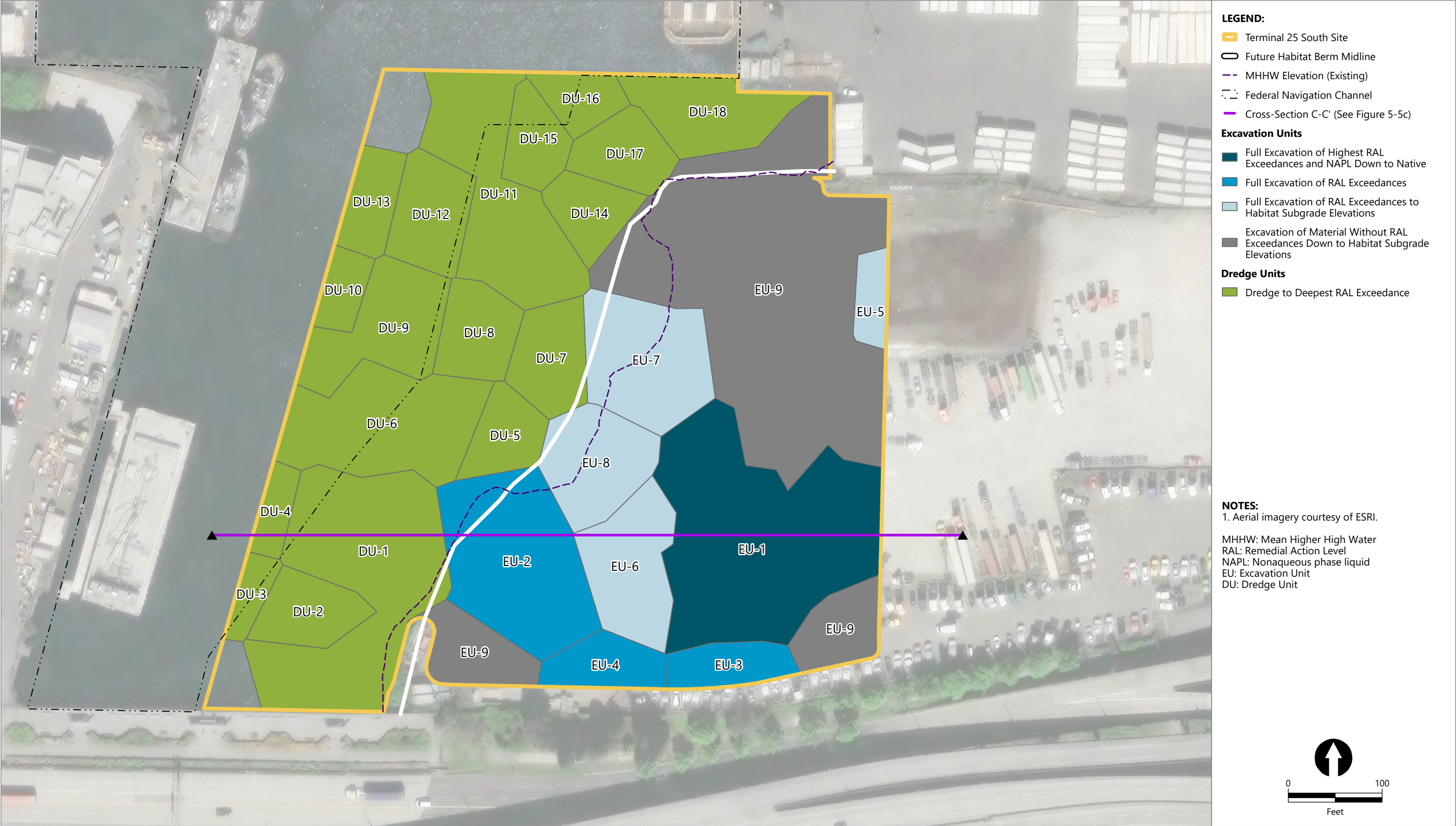
Figure 5-5a Alternative 3 Removal - Plan View Engineering Evaluation and Cost Analysis Terminal 25 South Site
