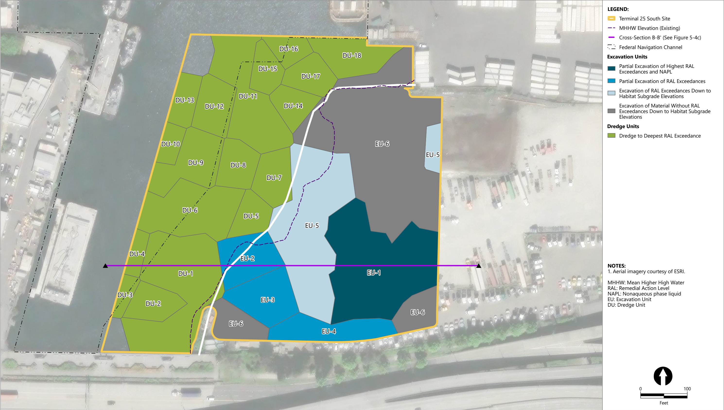
Figure 5-4a Alternative 2 Removal - Plan View Engineering Evaluation and Cost Analysis Terminal 25 South Site
