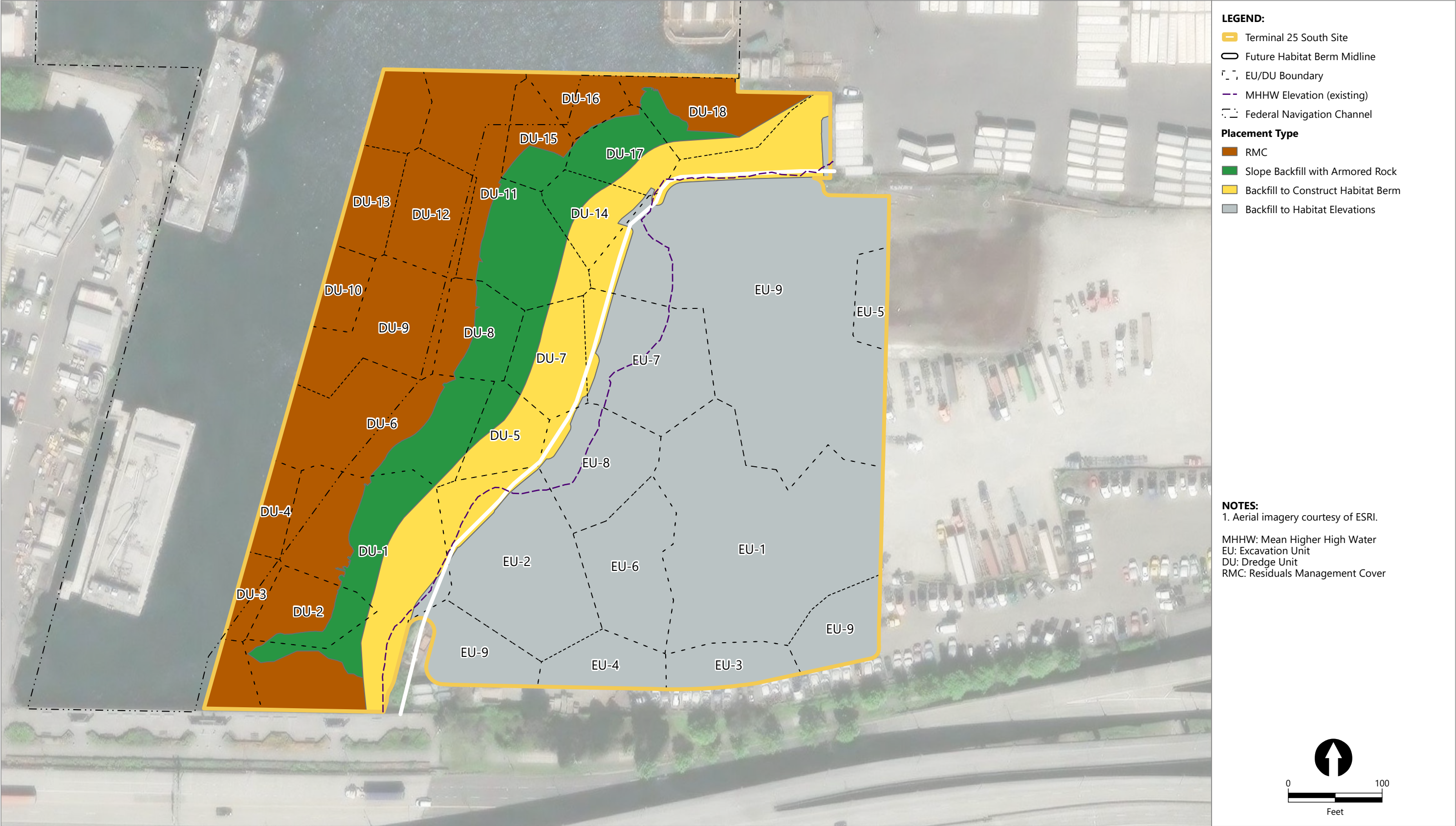
Figure 5-5b Alternative 3 Placement - Plan View Engineering Evaluation and Cost Analysis Terminal 25 South Site
