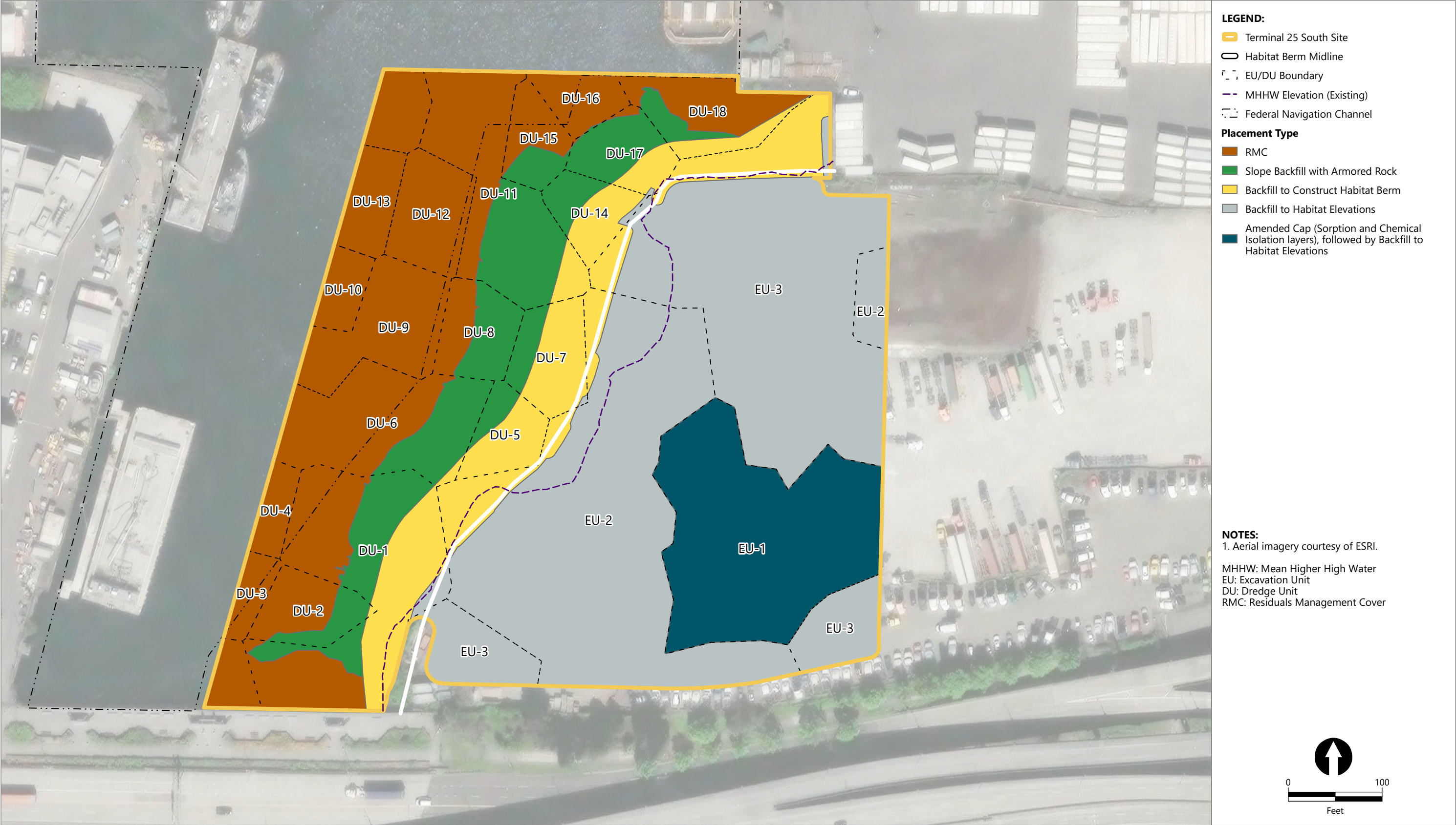
Figure 5-3b Alternative 1 Placement- Plan View Engineering Evaluation and Cost Analysis Terminal 25 South Site
