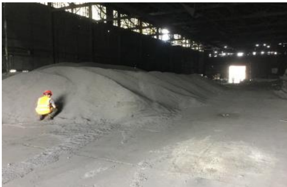
Figure 3: "Green coke" waste piles are one of several primary sources containing high levels of carcinogenic PAHs migrating from the facility parcel through the stormwater system and found at elevated concentrations in settling ponds.
