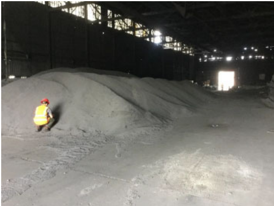
Figure 6: "Green coke" waste piles containing high levels of carcinogenic PAHs. One example of uncontrolled waste material.
