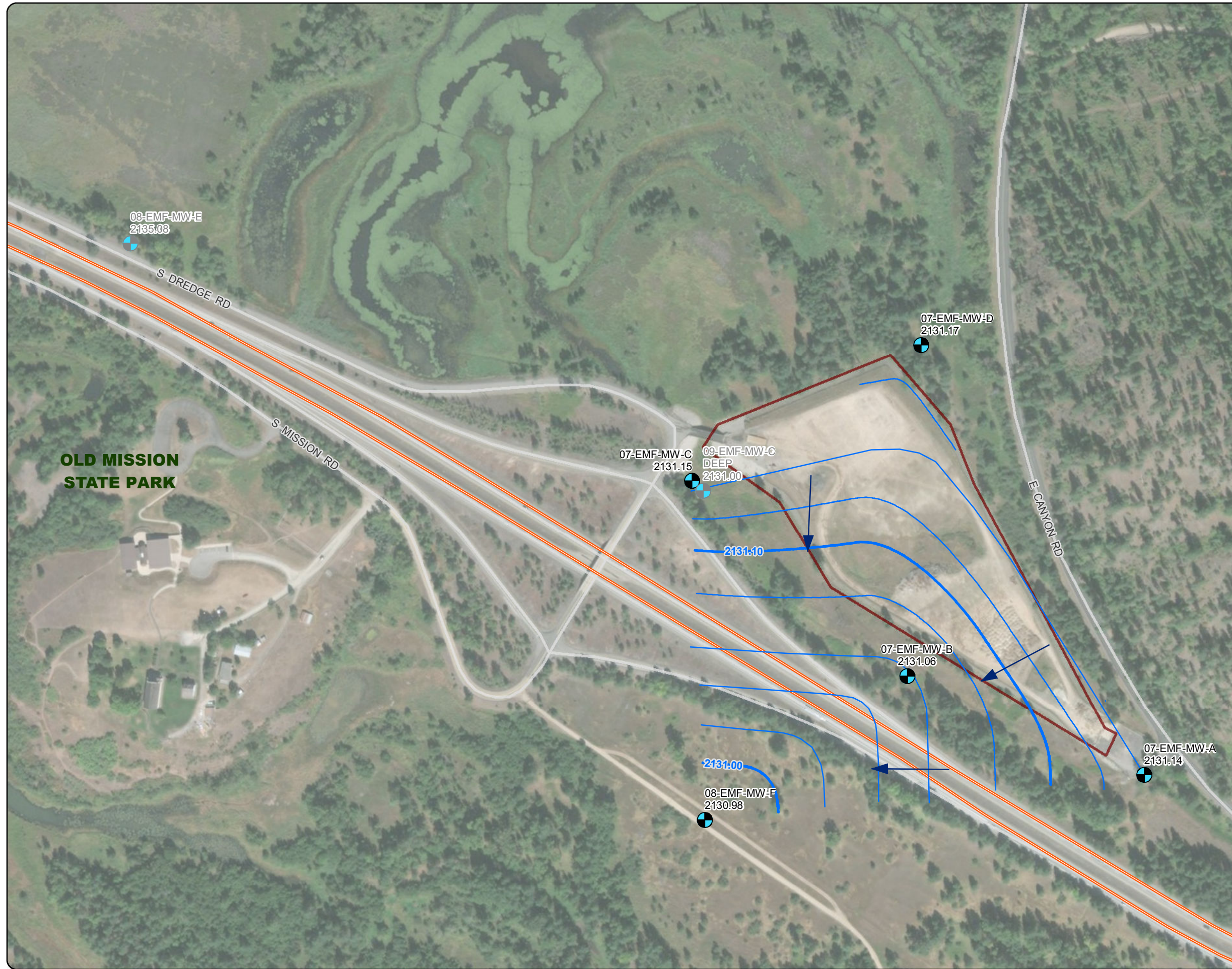
Figure 4-4 October 2017 Groundwater Potentiometric Surface Contours
