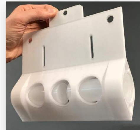
Porewater peeper sampling device Source: Geosyntec
