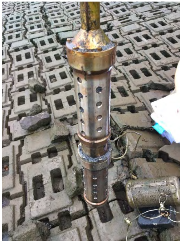
Photograph 7 – Recovered sub-armoring, inter-armoring, and surface water sampler from early warning sample location number 12 during September 2015 sediment cap performance monitoring.
