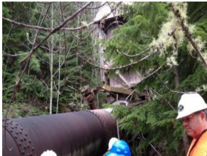
Photo 4a. Structure associated with a mill furnace. 4b. Rotary kiln and mill. Note mercury vapor capture device installed at left side of building.
