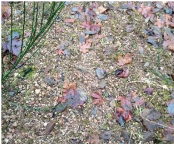
Photo 4. Mine tailings pile (notice the different tailing sizes from larger gravel to fines). Tailings are materials left over after the process of separating the valuable minerals from the ore.
