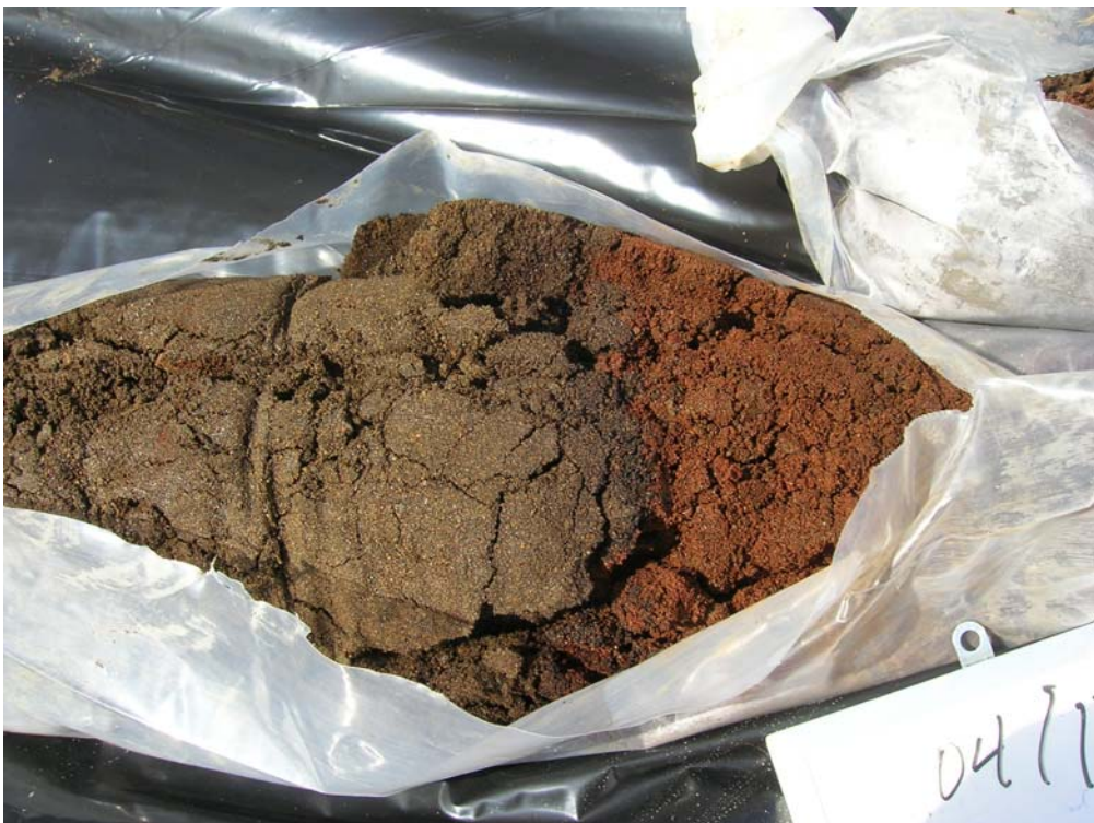
Photograph 14 – Representative lithology: color change in well-graded sand (SW) collected from SC0111 (5-7.5 feet bgs)
