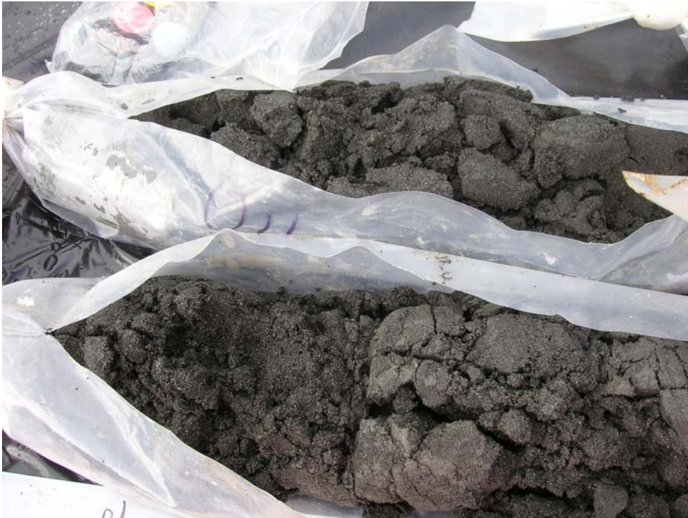
Photograph 15 – Representative Lithology: poorly graded sand (SP) collected from SC0111 [105-100 feet bgs (front) and 110-105 feet bgs(back)].
