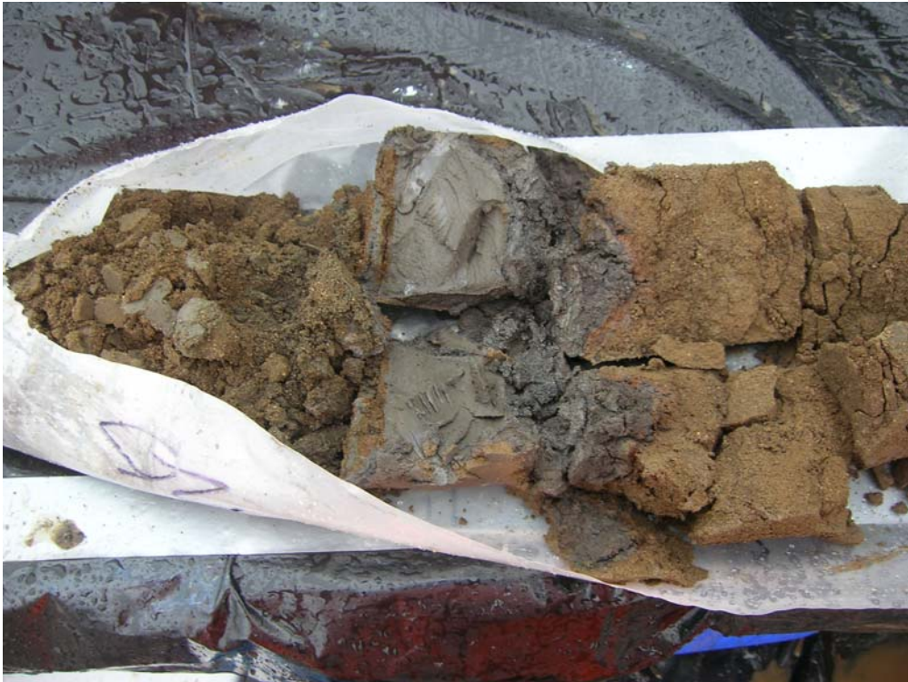
Photograph 17 – Silt layer observed 19-19.5 feet bgs in SC0411. Note the sheen and thin layer of staining on the upper (right) side of the silt layer.
