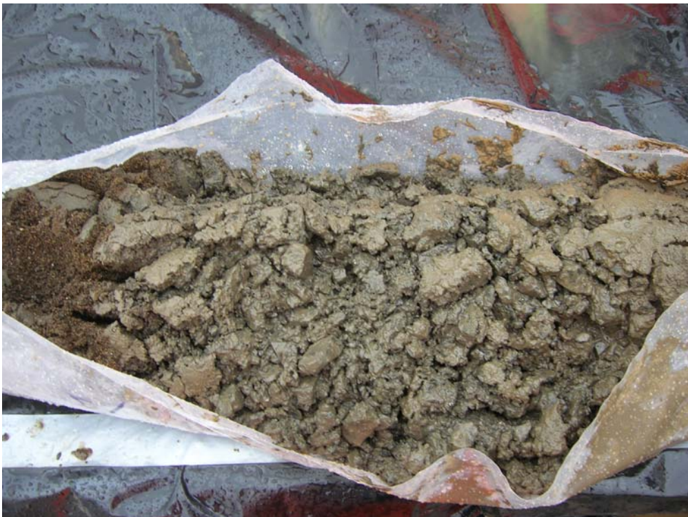
Photograph 16 – Well-graded gravel observed 11 to 14.5 feet bgs in SC0411.
