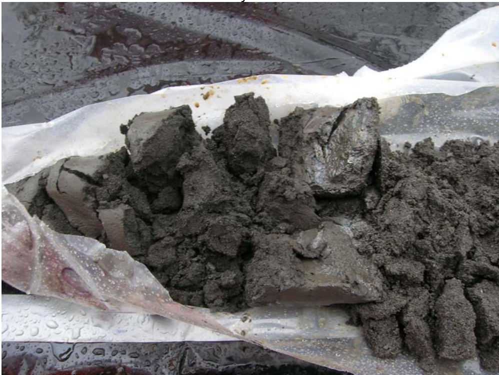
Photograph 18 – Sheen and staining observed on top (right) of silty sand layer at 34 feet bgs in SC0311.
