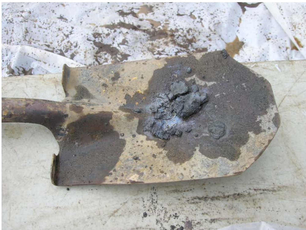
Photograph 19 – Sheen and staining observed in poorly graded sand (SP) at a depth of approximately 95 feet bgs in SC0211.
