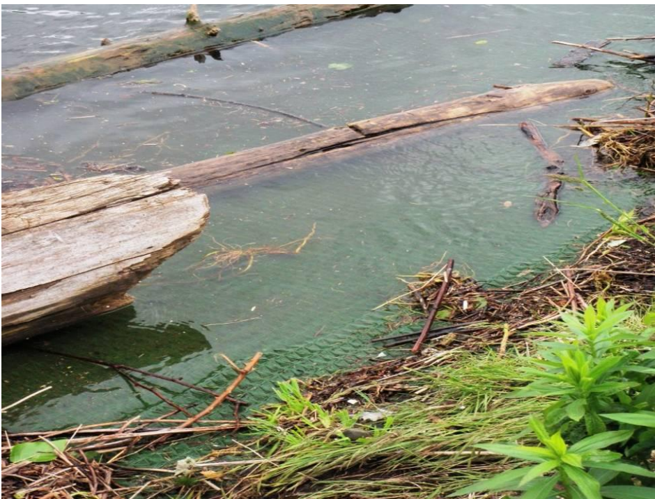
Photograph 2 – Erosion matting exposed due to high water (June 2011).
