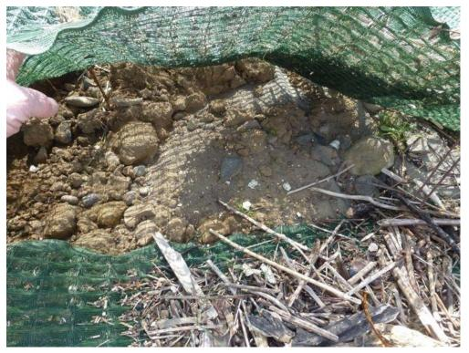
Photograph 1 - Eroded soil observed under the TRM.
