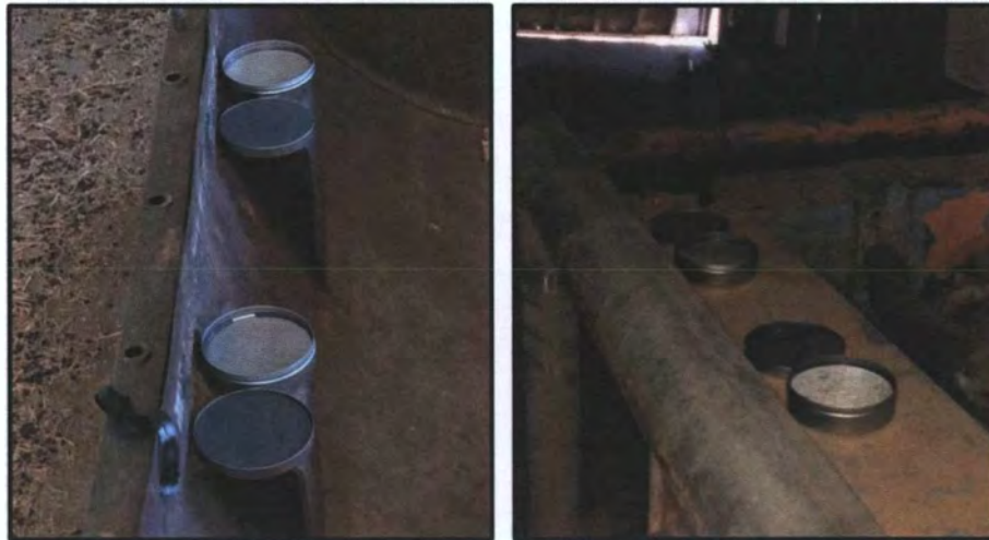
Figure 6: Short-term radon test kits as deployed in the west building (left) and east building (right) at the Mac No. 1 Mine Site.
