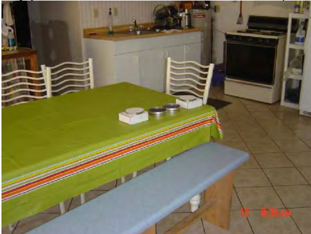
Photo 3: Indoor air radon canister sampling.
