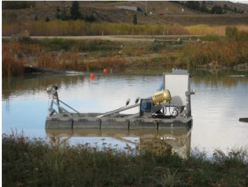
BPSOU: Butte Treatment Lagoons dredging equipment in B series
