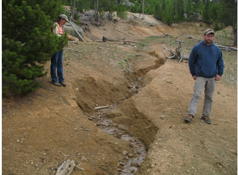
PHOTOGRAPH 1-3. Erosion Rill Formed through Former Waste Rock Dump Location
