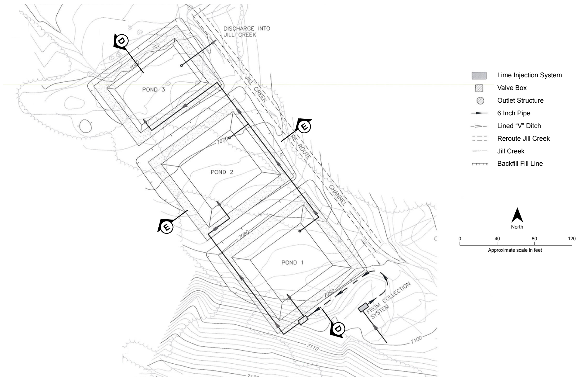
FIGURE 3-7 BULLION SEMI-ACTIVE TREATMENT Bullion Mine Feasibility Study
