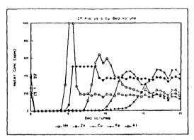
Fig 3 — Selective desorption of metals.
