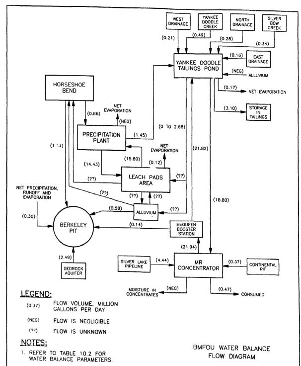
2. FLOW FROM McQUEEN BOOSTER STATION INTO BERKELEY PIT EQUALS 0.14 MGD OF SLURRY OR 0.12 MGD OF WATER ONLY.
