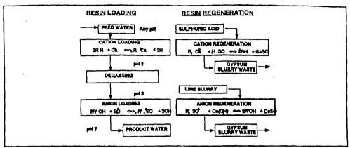
Figure 1 GYP-CIX PROCESS CHEMISTRY
