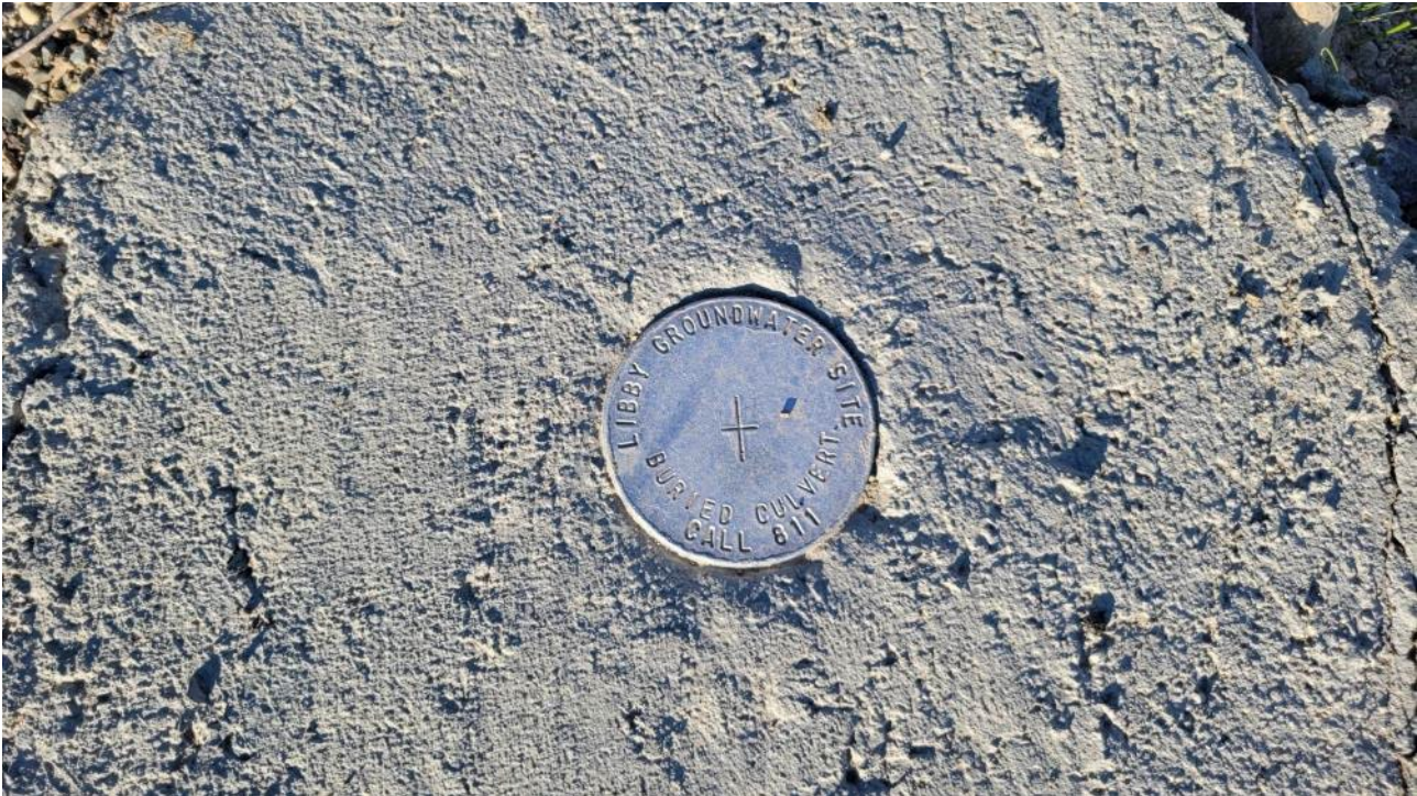
Photograph 18: Area 2 ISB utility marker installed for future development changes to planned new road.
