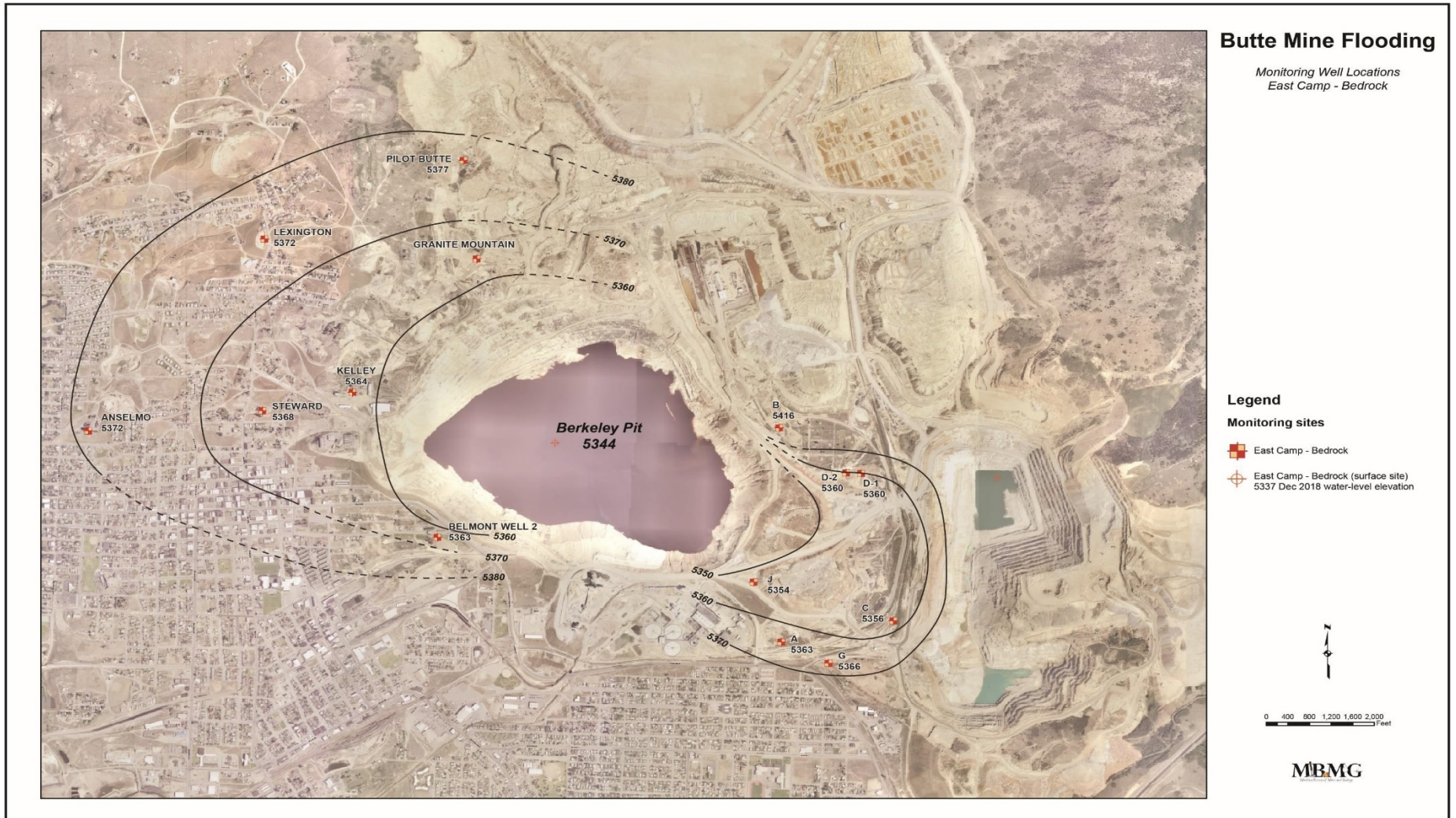
Figure 3-15. Potentiometric map for the East Camp bedrock aquifer, December 2018 (contour interval is 10 ft).
