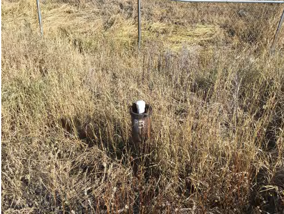
Peizometer P3 showing the casing extending above the casing. The casing was cut on 10/16 to allow the lid to be securely fastened. See photo below after work was completed.
