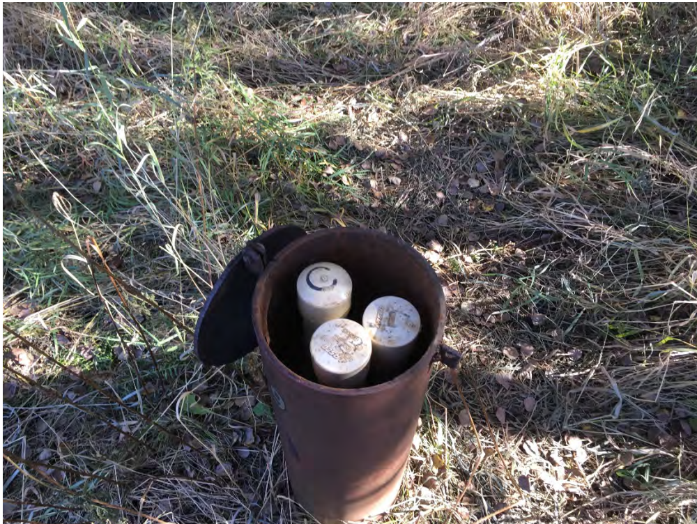
Wells 9A, B and C without a lock. Photo taken on 10/16. This was discussed with the site operator who said that a lock would be placed on the well that day. Photo below shows inside casings.
