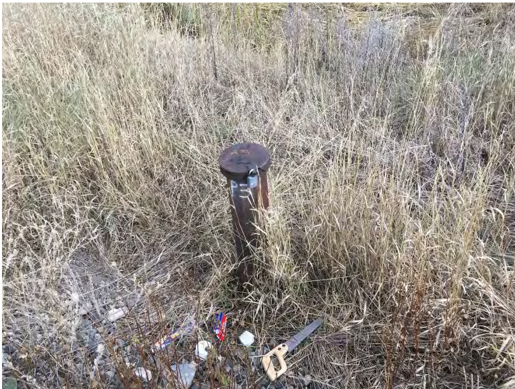
Peizometer P3 showing the casing extending above the casing. The casing was cut on 10/16 to allow the lid to be securely fastened. See photo below after work was completed.
