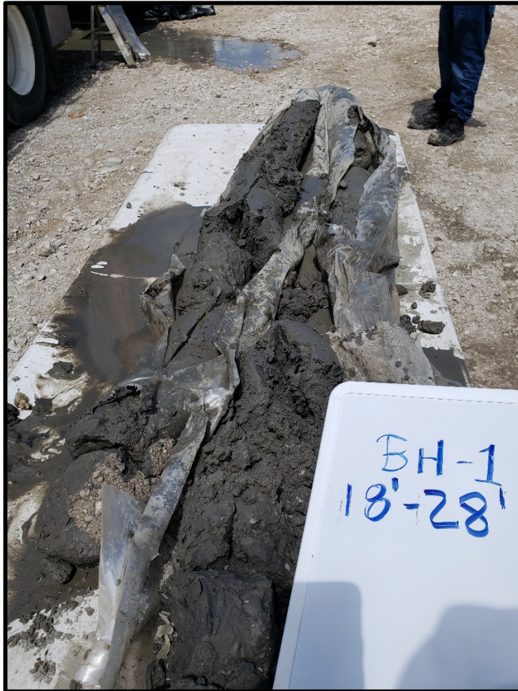
PHOTOGRAPH NO. 6 Returned materials from 18 feet to 28 feet in Borehole BH-1.
