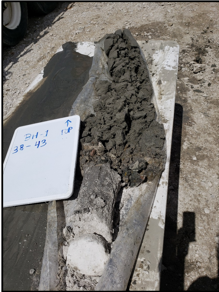
PHOTOGRAPH NO. 8 Materials returned from 38 feet to 43 feet in Borehole BH-1.
