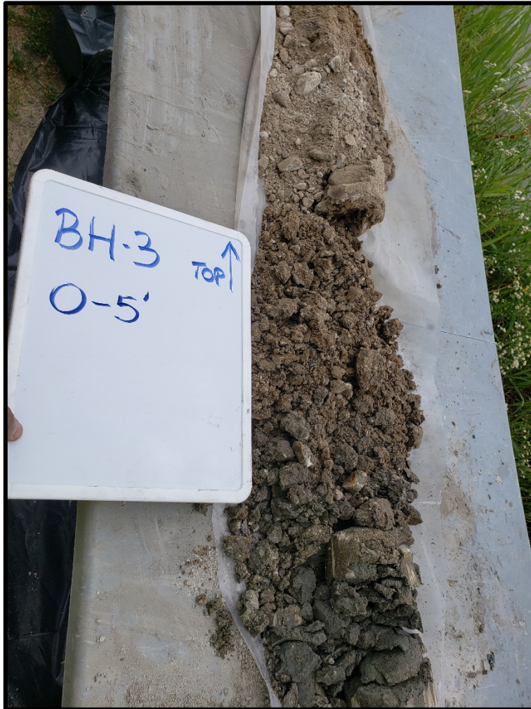
PHOTOGRAPH NO. 19 Materials returned from 0 feet to 5 feet in Borehole BH-3.
