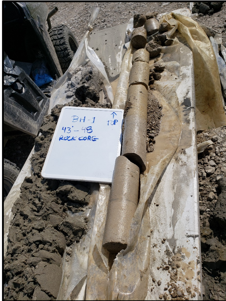
PHOTOGRAPH NO. 9 Rock core from 43 feet to 48 feet in Borehole BH-1.
