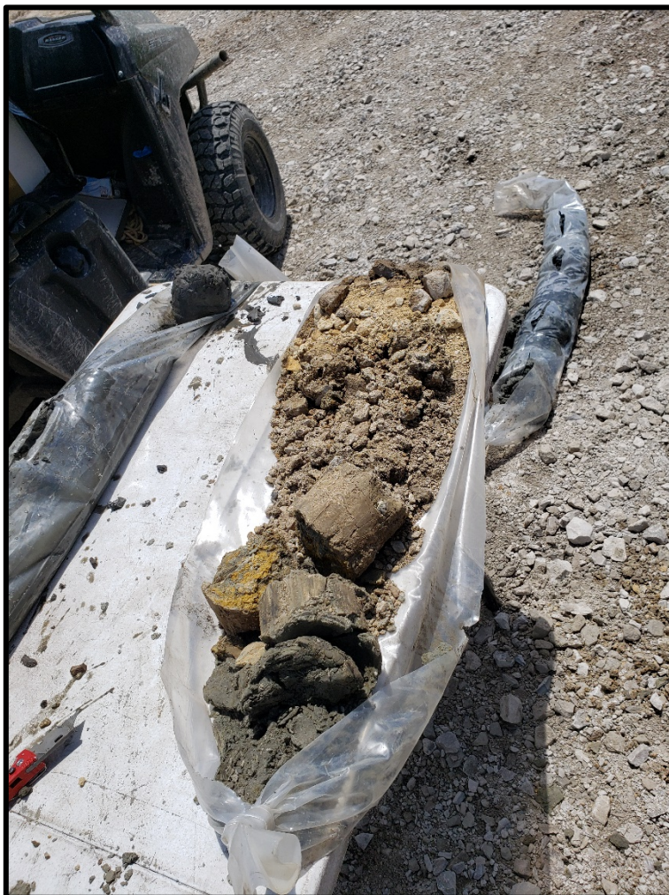
PHOTOGRAPH NO. 3 Materials returned from 0 feet to 5 feet in Borehole BH-1.
