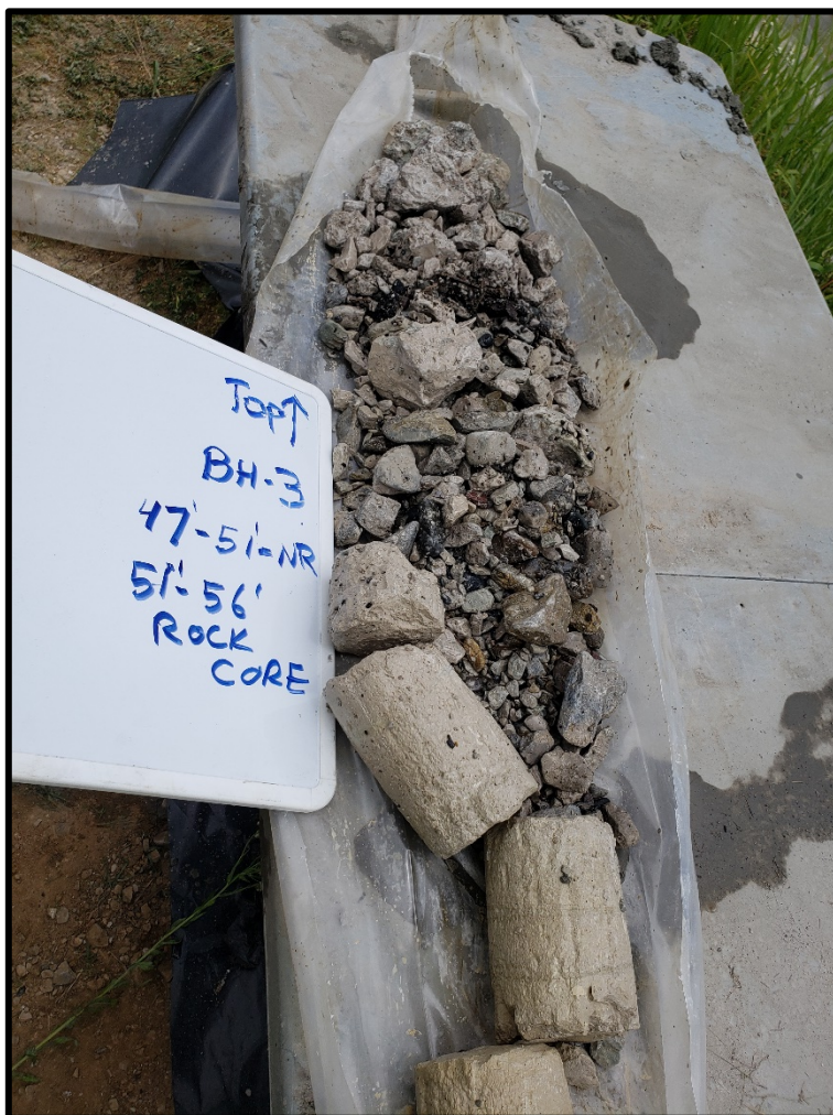
PHOTOGRAPH NO. 25 Rock core from 51 feet to 56 feet in Borehole BH-3.
