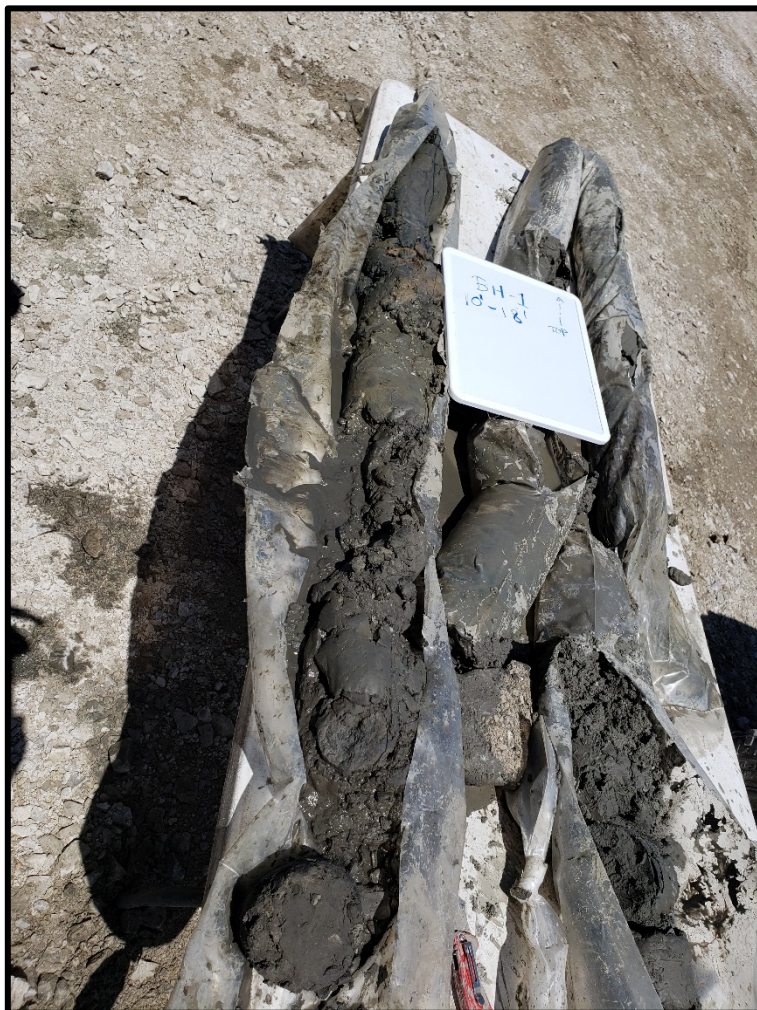
PHOTOGRAPH NO. 5 Materials returned from 10 feet to 18 feet in Borehole BH-1.
