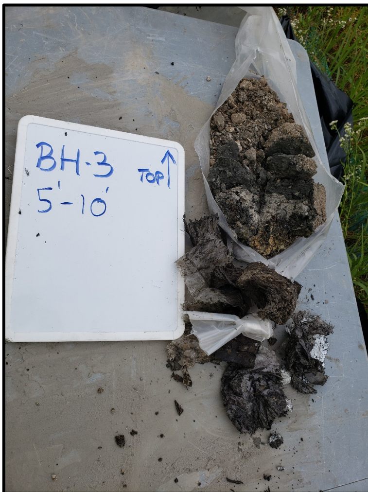
PHOTOGRAPH NO. 20 Materials returned from 5 feet to 10 feet in Borehole BH-3.
