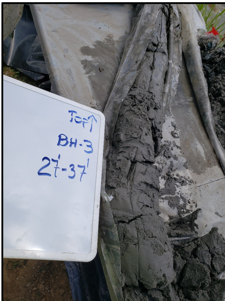
PHOTOGRAPH NO. 23 Materials returned from 27 feet to 37 feet in Borehole BH-3.
