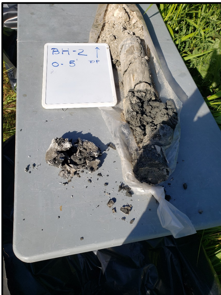
PHOTOGRAPH NO. 10 Returned materials from 0 feet to 5 feet in Borehole BH-2.
