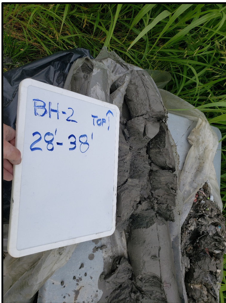
PHOTOGRAPH NO. 15 Returned materials from 28 feet to 38 feet in Borehole BH-2.
