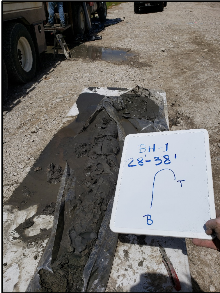
PHOTOGRAPH NO. 7 Materials returned from 28 feet to 38 feet in Borehole BH-1.
