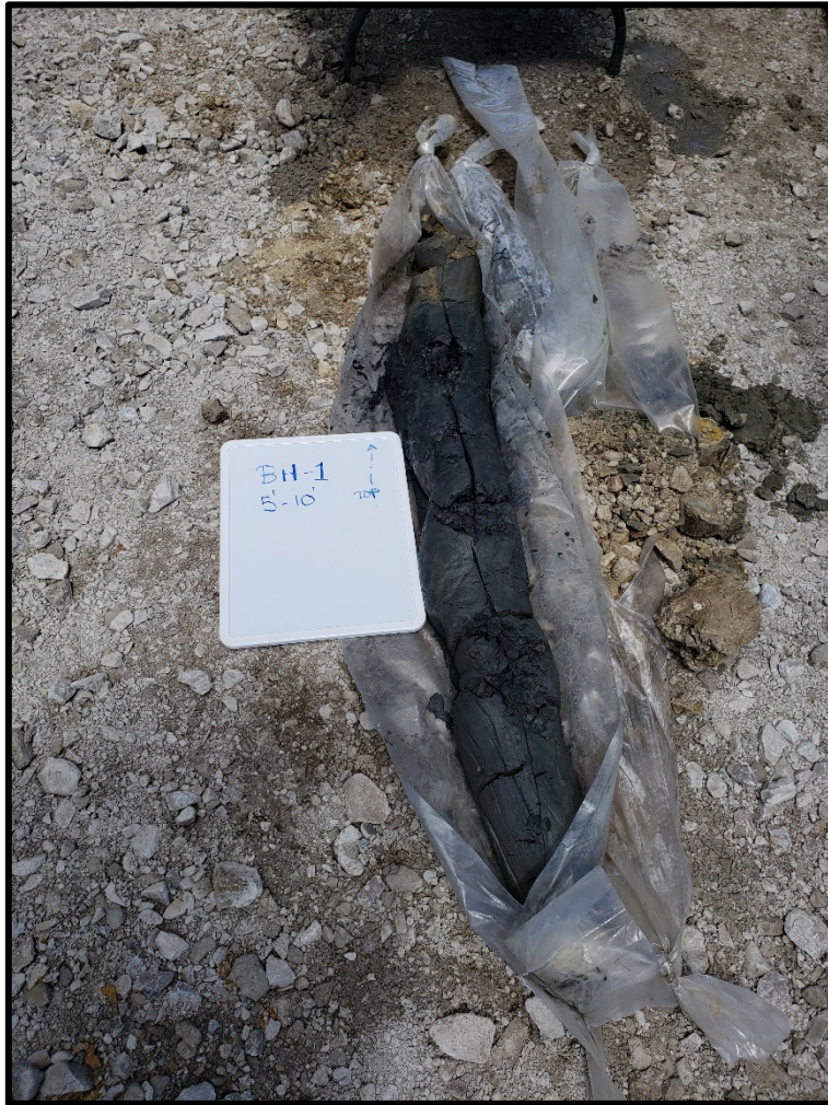
PHOTOGRAPH NO. 4 Returned materials from 5 feet to 10 feet in Borehole BH-1.
