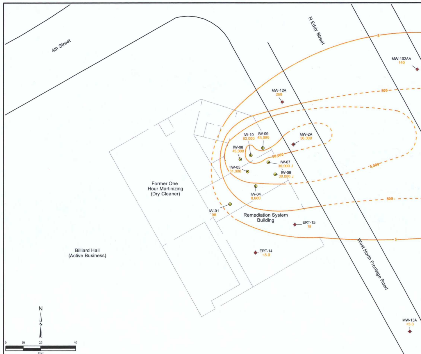
Figure 4-8 PCE Isoconcentrations OU2 Source Area July 2015 (Upper Portion of the Aquifer)
