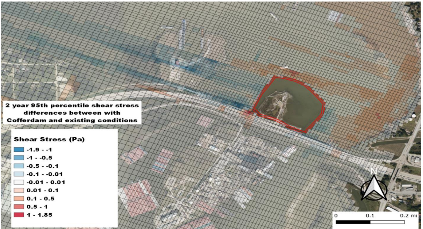
Figure 24 95 th Percentile Shear Stress Differences Between “With Cofferdam” and Existing Conditions for the 2-Year Storm
