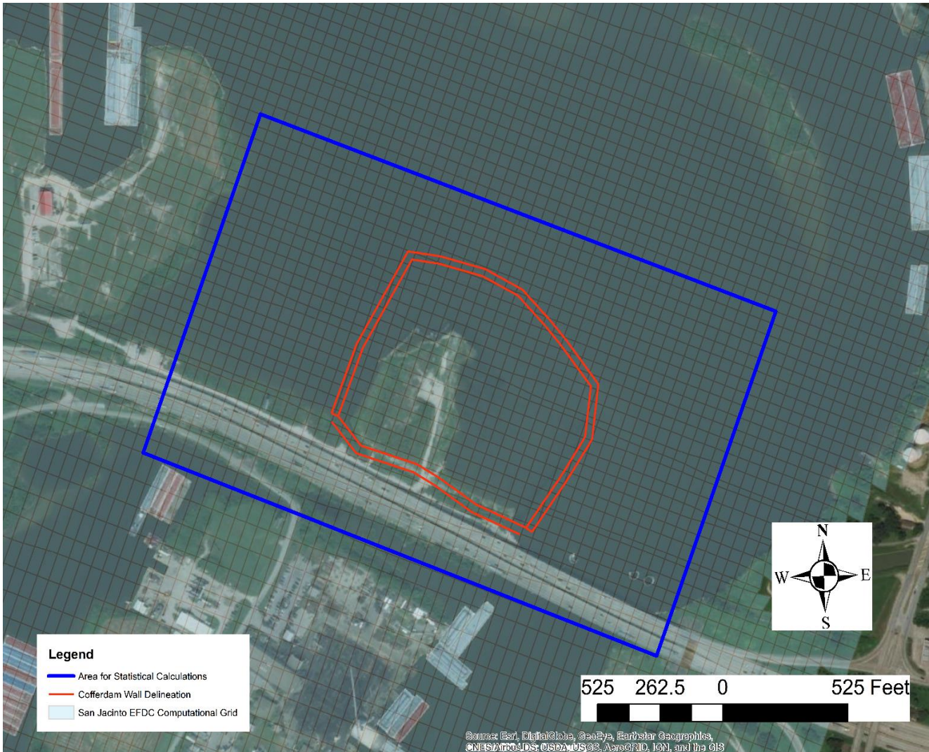
Figure 22 Area Used for the Computation of Statistics for the Conditions Around the Cofferdam
