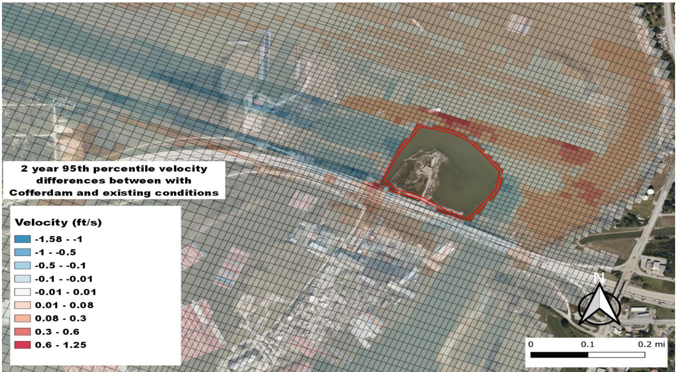
Figure 26 95 th Percentile Velocity Differences Between “With Cofferdam” and Existing Conditions for the 2-Year Storm
