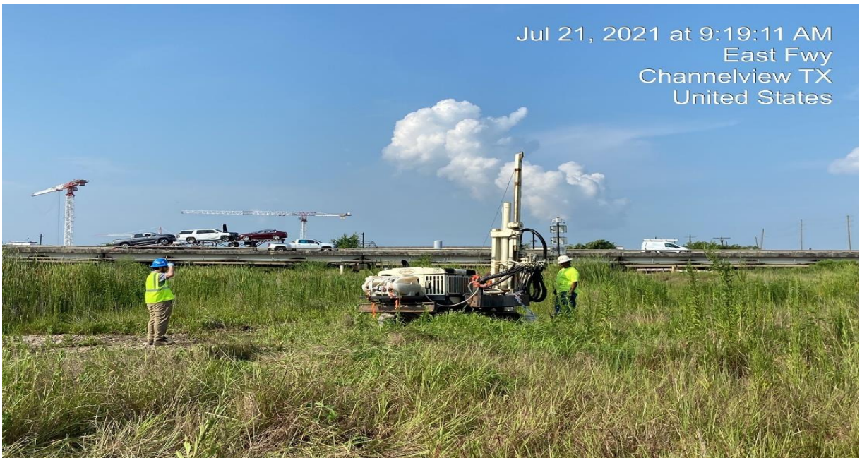
Photo 4 Drill crew positioning a geoprobe drilling rig at boring location SJSB078.
