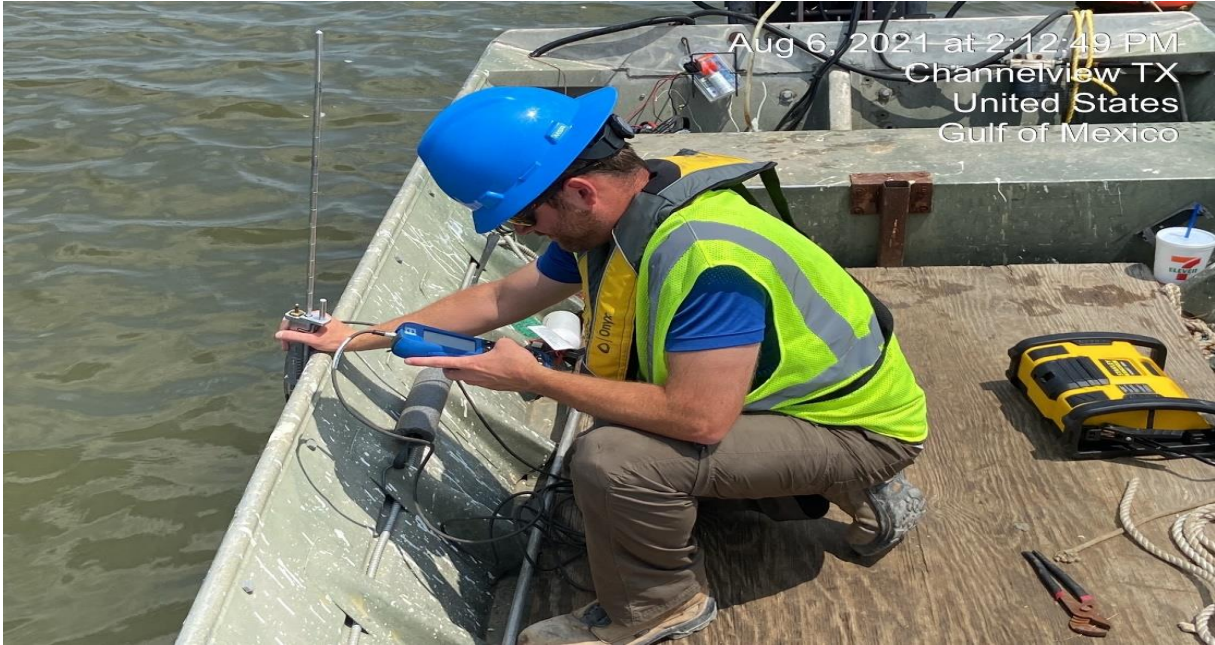
Photo 11 GHD personnel collecting water velocity measurements near the turbidity curtain.
