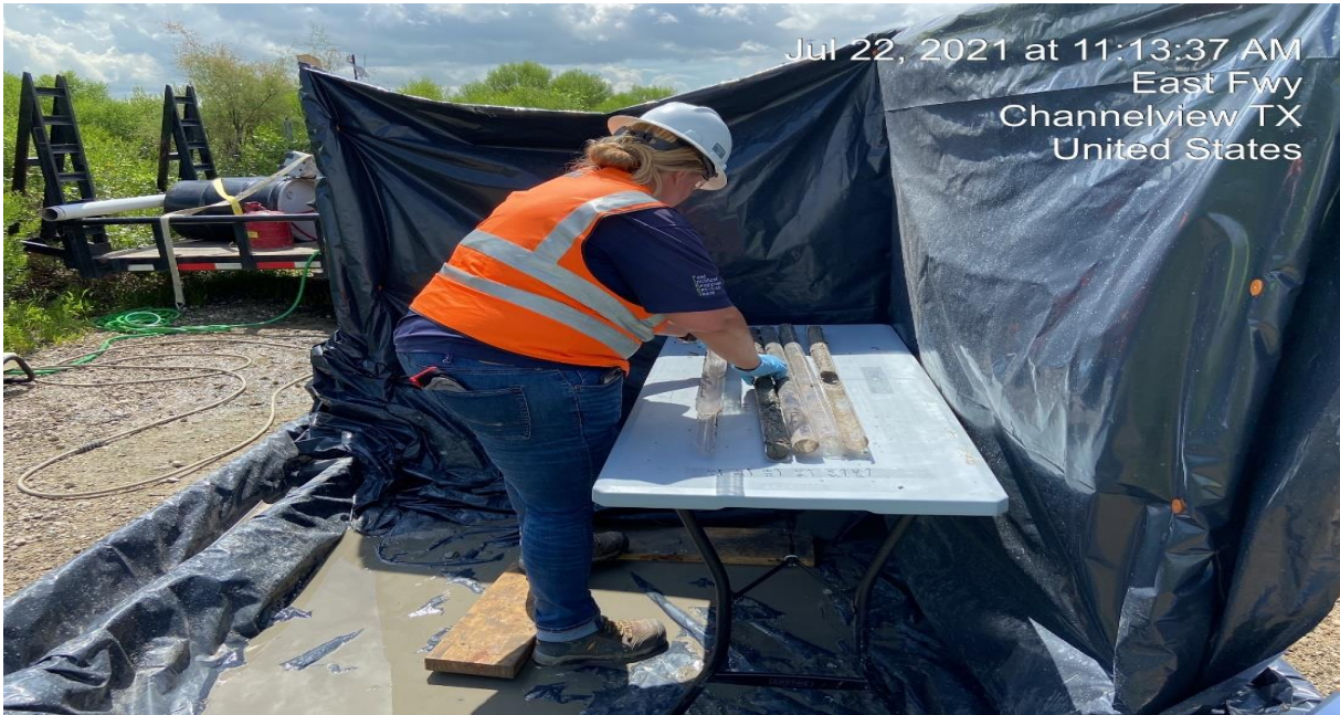
Photo 5 GHD personnel logging soil cores and collecting samples from boring SJSB083.
