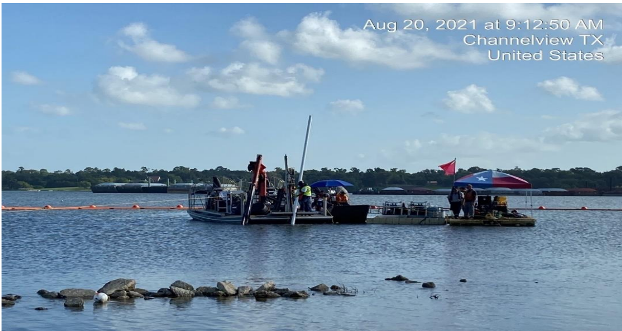
Photo 16 View from land, airboat drilling crew collecting soil cores from boring location SJSB098.
