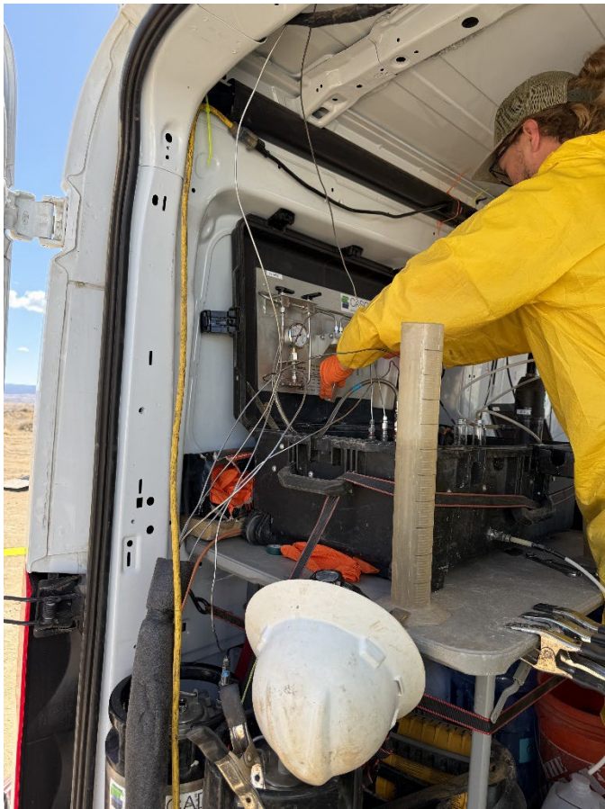
Photo 4: Field Personnel Collecting Discrete Level Groundwater Sample using the Waterloo Profiler
