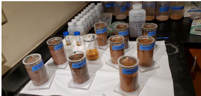
Photo 5: Soil cores from the 7 transects getting prepped in the lab for column testing
