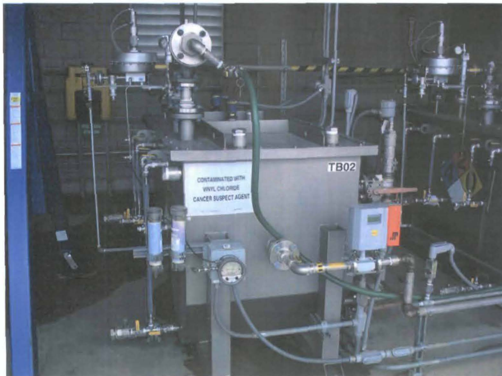
Photo 8. DNAPL/LNAPL separator for groundwater extraction wells in Hub Facility "B". Separator for DNAPL wells located to the right.
