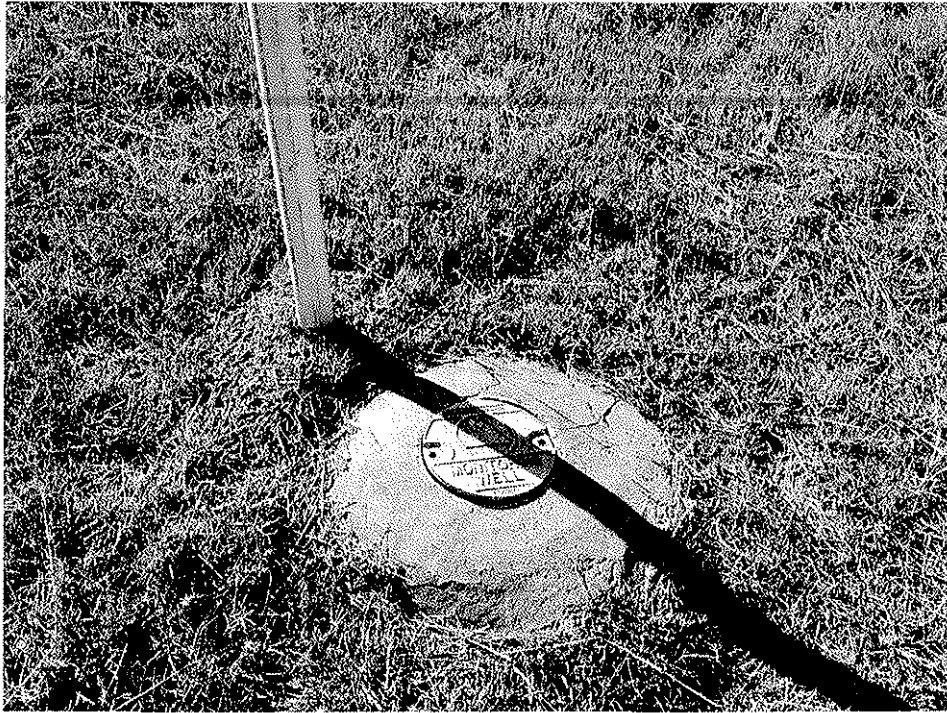
Typical Piezometer Surface Completion with ID Pipe
