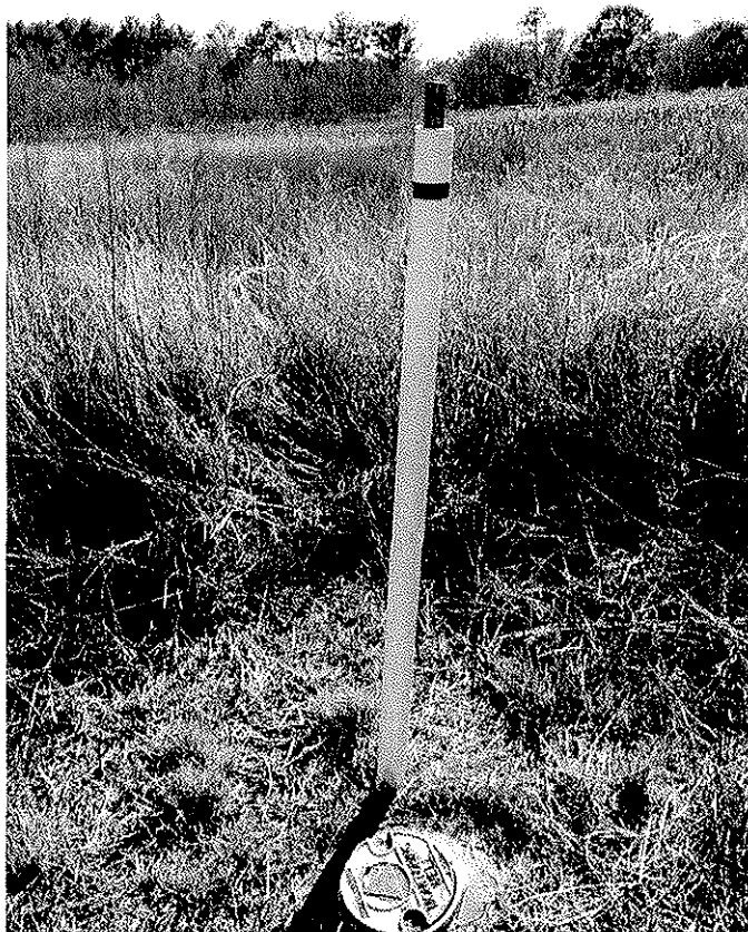
Typical Piezometer Surface Completion with ID Pipe
