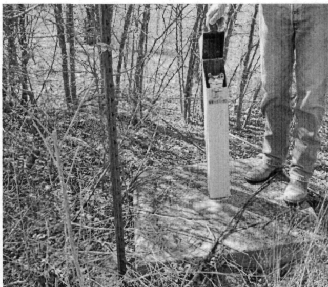
Photo 21. MW-33-90, well is missing the lock
