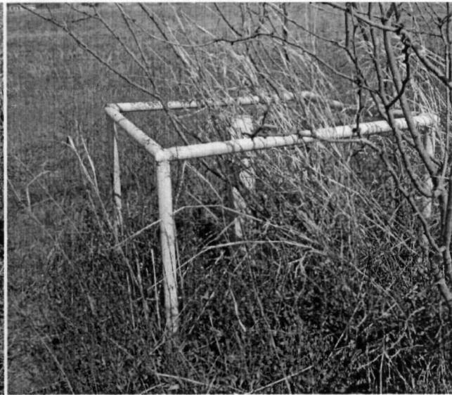
Photo 8. MW-17, has no identification marker, overgrown
