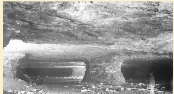
Room and pillar techniques made the mining possible. To remove the ore, large rooms – some with ceilings as high as 100 feet – were connected by horizontal tunnels known as drifts. Pillars were left within the rooms to support the ceilings.
