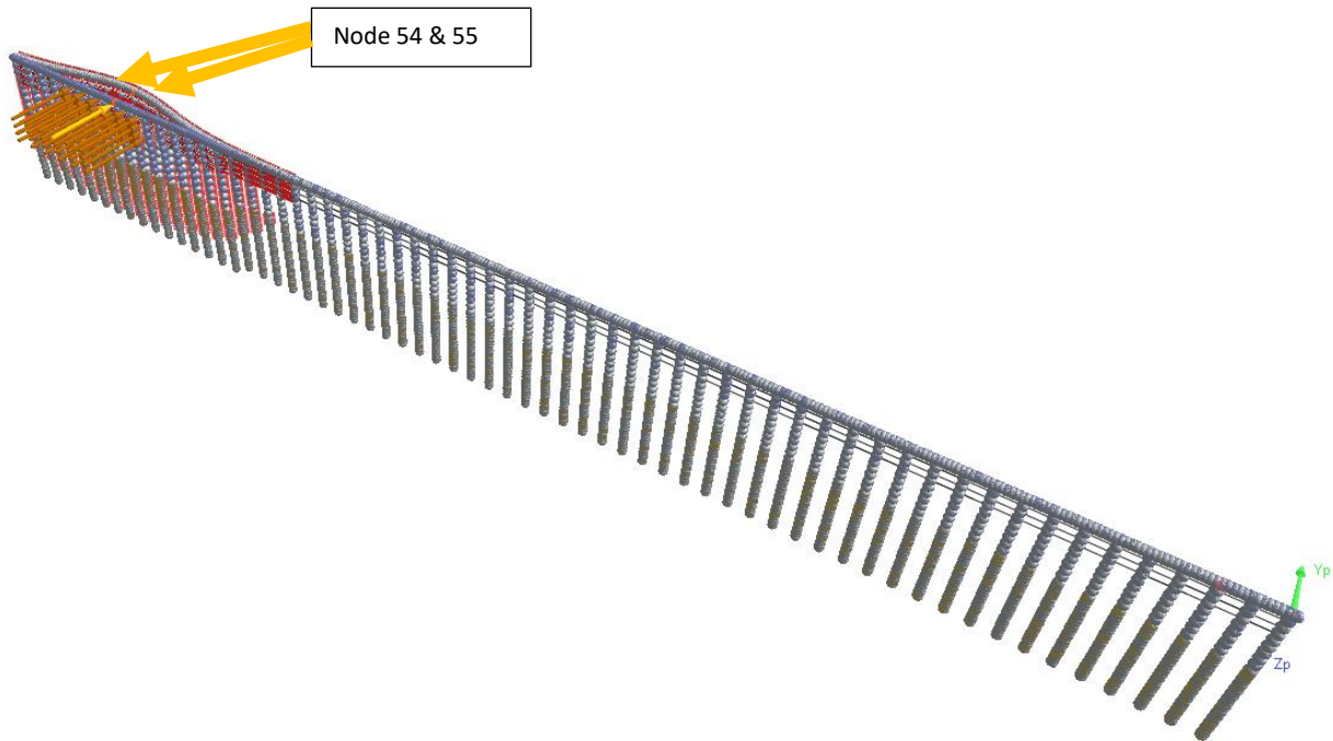
Figure 62: Displacement - Load Case 6 (Section 4 – Soil C5)
