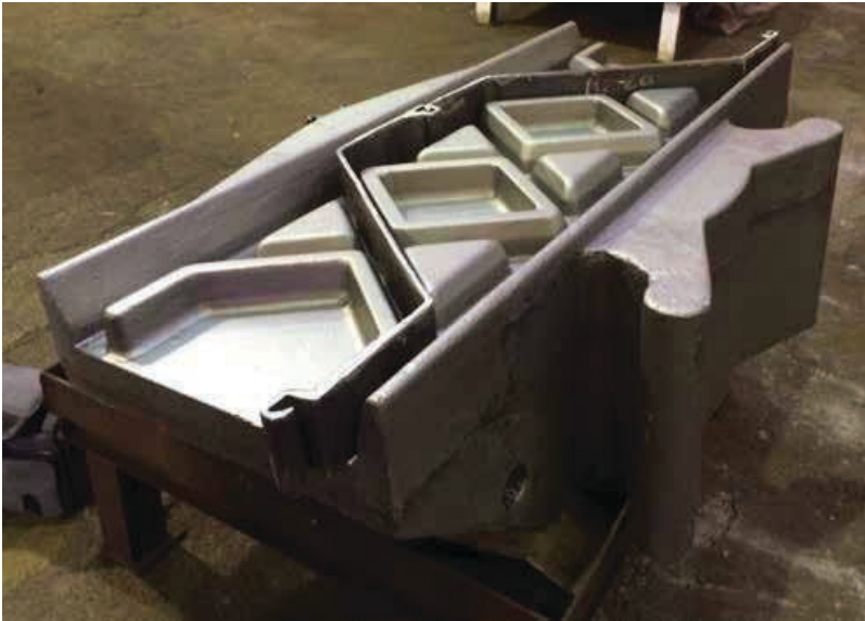
Typical driving cap for Z-sheet piles
