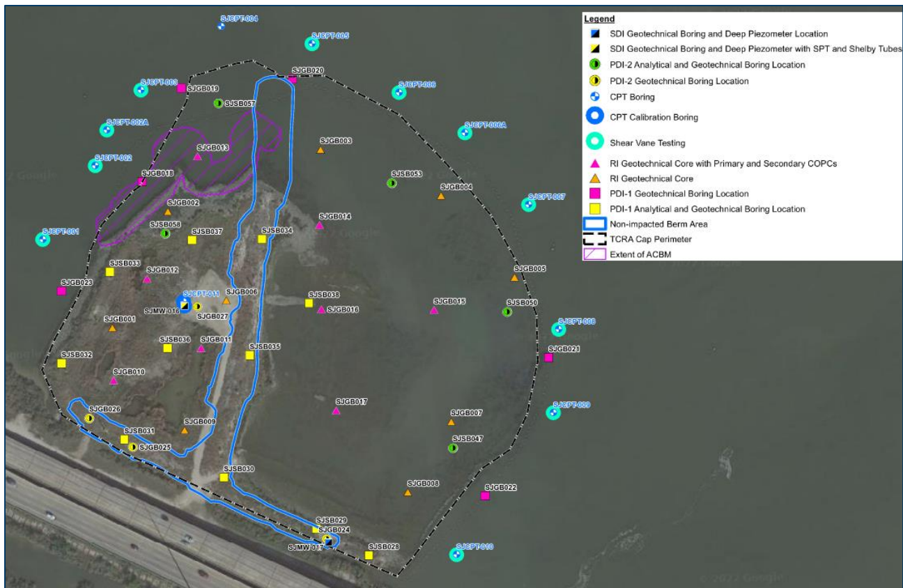
Figure 2.1 Locations of Geotechnical Soundings
