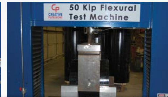
Bolted Connection Test - Perpendicular
