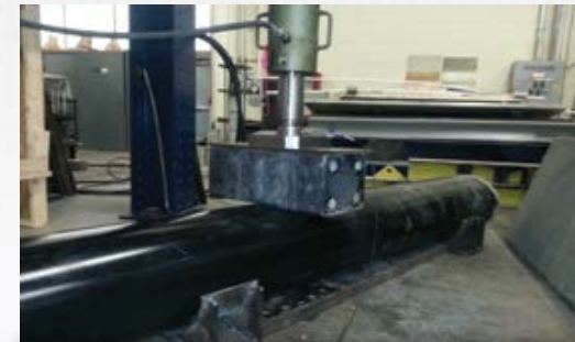
Crush Test on Concrete Filled Pile
