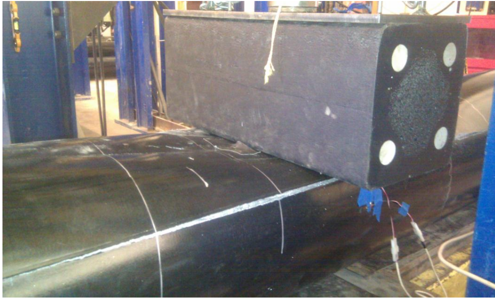
Figure 12: 16-inch Pile Failure Under Load
