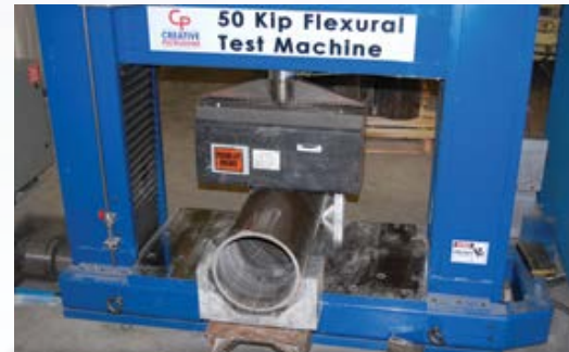
SUPERPILE® Crush Strength Test Set Up
