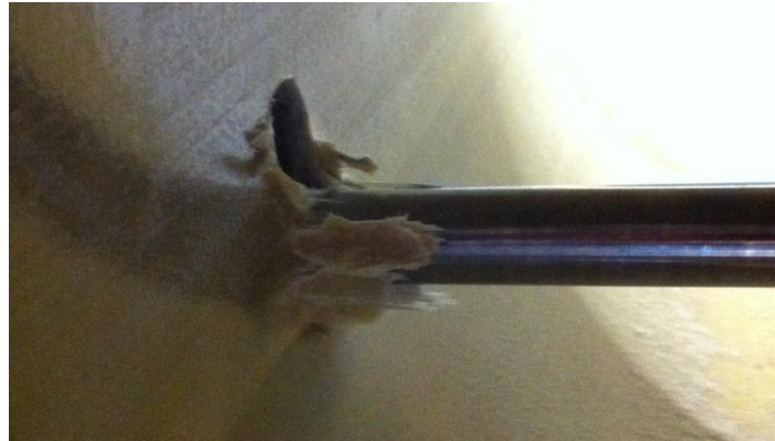
Figure 17: Typical Failure of Connection Test A
