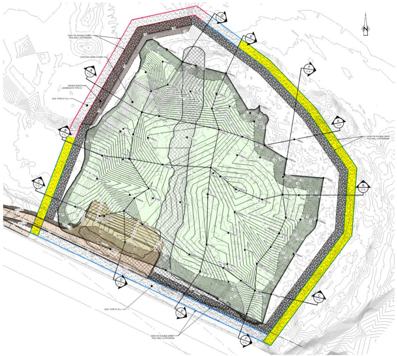
Figure 2: Eastern and western areas of the cofferdam, where a 55-ft grouted riprap apron and a 10-ft loose riprap apron is recommended (for river WSE=14 ft).
