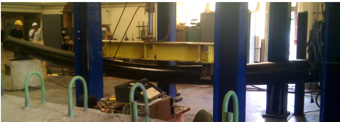
Figure 2: Four-Point Bending: 16-inch sample
