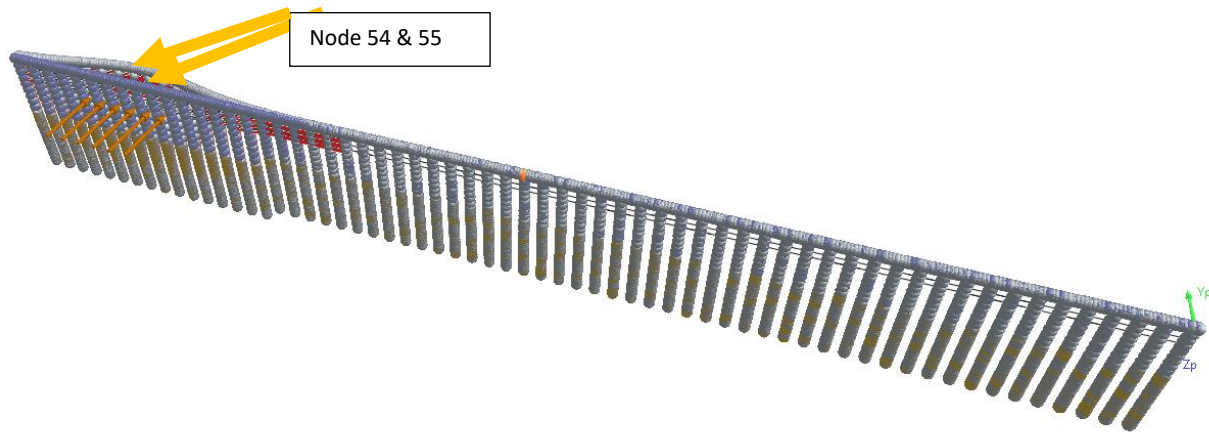
Figure 92: Displacement - Load Case 12 (Section 4-Soil C5)
