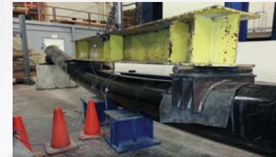
Full Section Testing of Concrete Filled Pile
