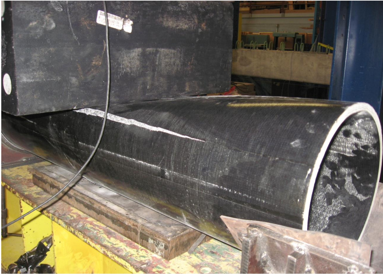
Figure 10: 12-inch Crush Test Pile Failure
