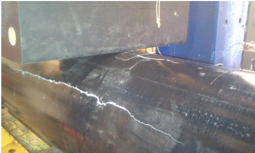
Figure 13: 16-inch Pile at Failure with Load Released
