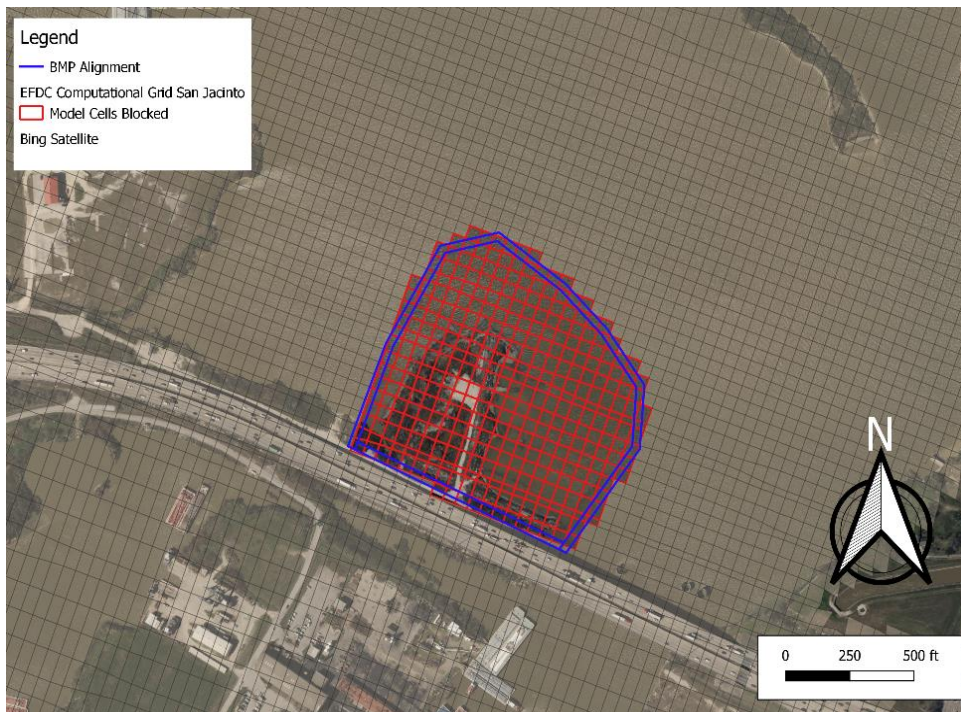
Figure 10 Model Grid Showing Delineation of Cofferdam and Cell Models Defining the Northern Impoundment
