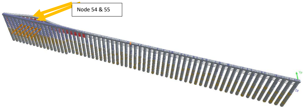
Figure 92: Displacement - Load Case 12 (Section 4-Soil C5)
