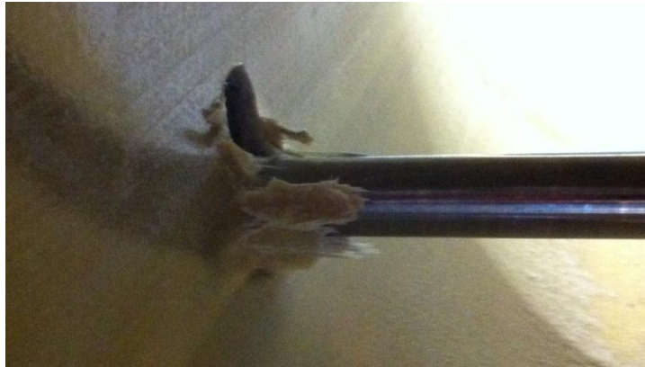
Figure 17: Typical Failure of Connection Test A
