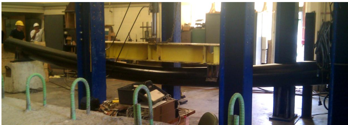
Figure 2: Four-Point Bending: 16-inch sample
