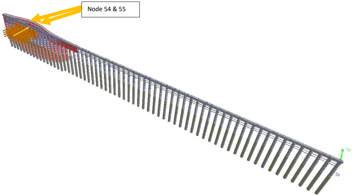
Figure 62: Displacement - Load Case 6 (Section 4 – Soil C5)
