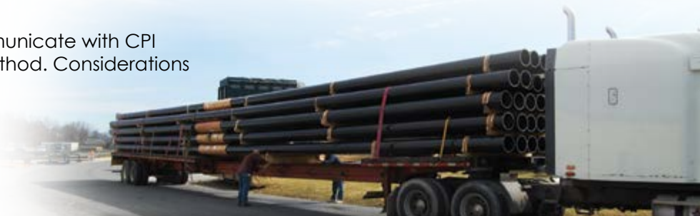
Dedicated Truck Hauling 80' Piles to Margate, New Jersey
