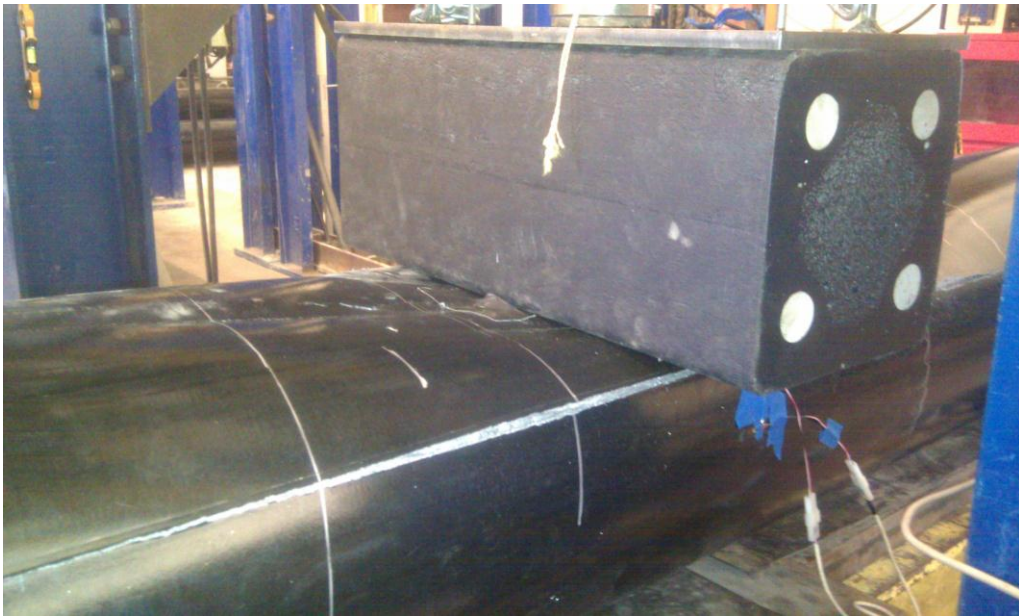
Figure 12: 16-inch Pile Failure Under Load
