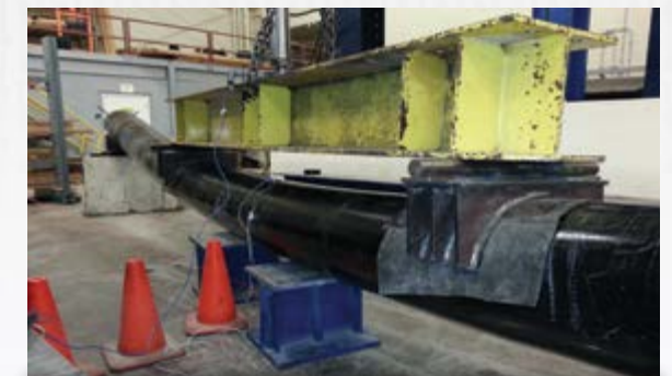
Full Section Testing of Concrete Filled Pile
