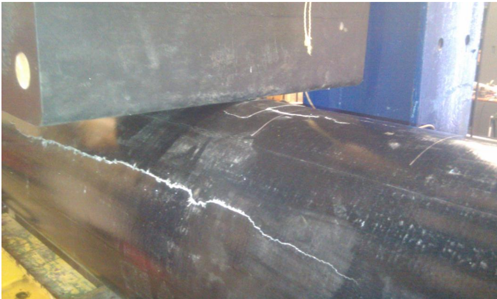
Figure 13: 16-inch Pile at Failure with Load Released
