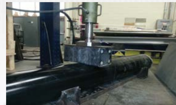
Crush Test on Concrete Filled Pile
