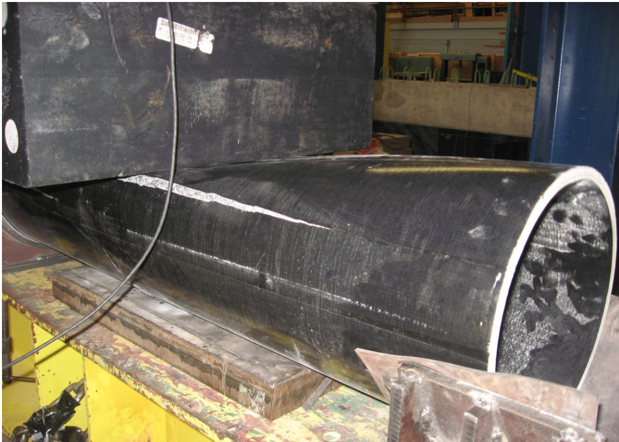
Figure 10: 12-inch Crush Test Pile Failure
