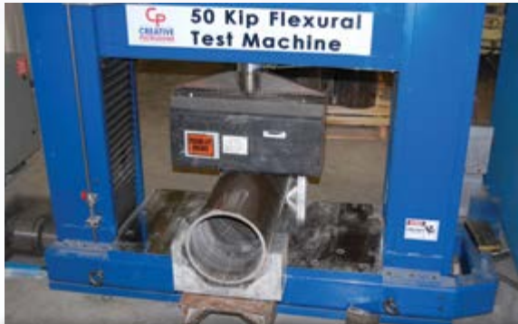
SUPERPILE® Crush Strength Test Set Up
