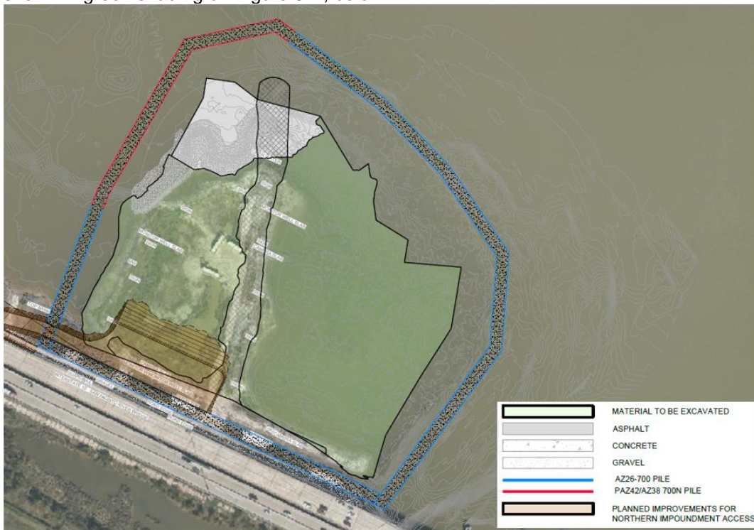
Figure 5-B BMP Alignment and Excavation Extent
