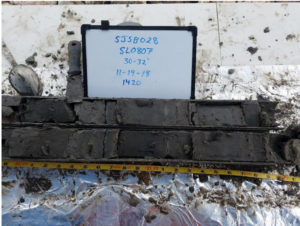
Photo 15 - Geotechnical Sample SJSB028 (30-32)
