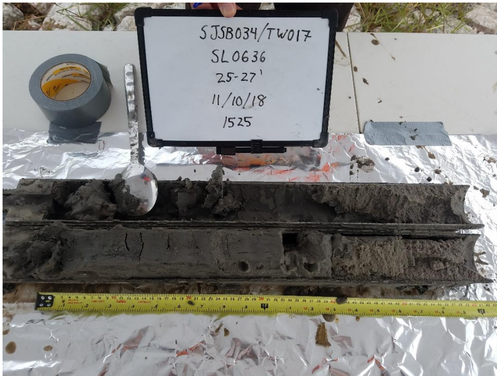
Photo 40 - Geotechnical Sample SJSB034 (25-27)
