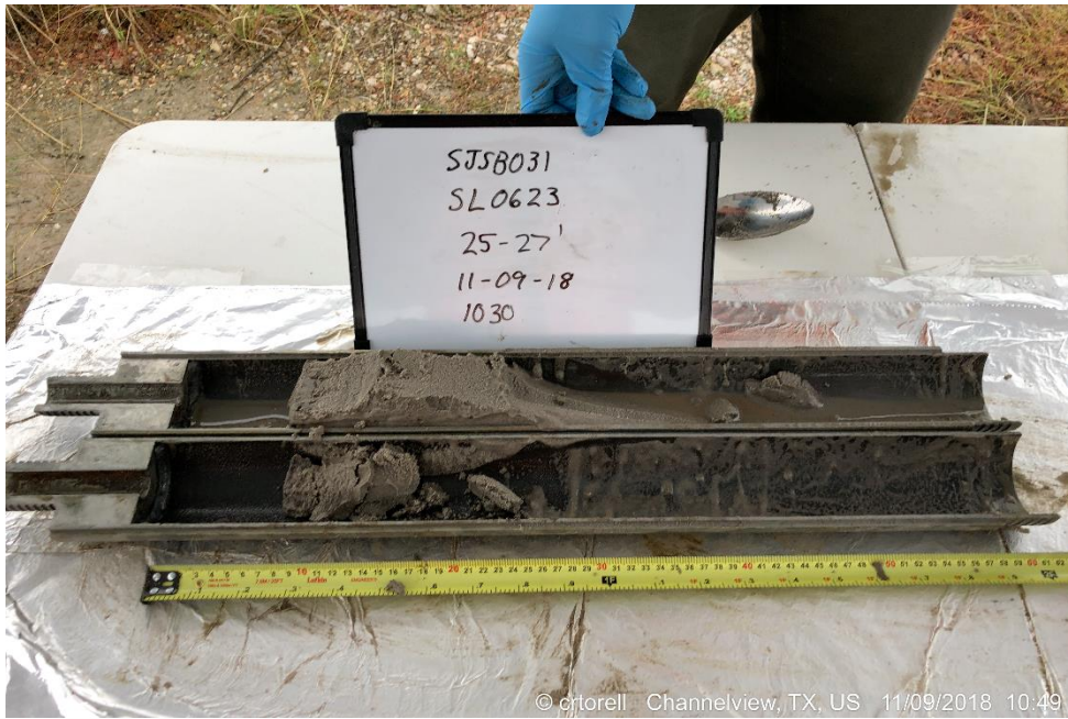
Photo 27 - Geotechnical Sample SJSB031 (25-27)
