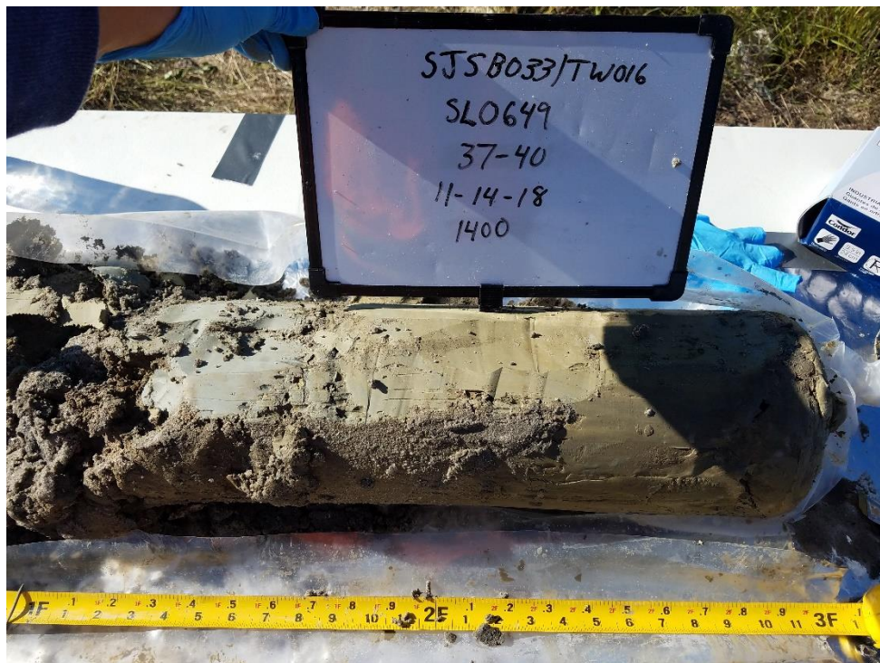
Photo 36 - Geotechnical Sample SJSB033 (37-40)
