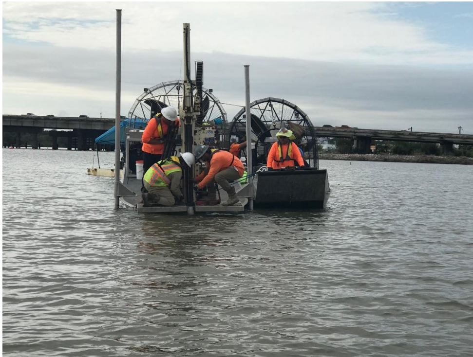
Photo 3 - Drill crew working from airboats, collecting samples.
