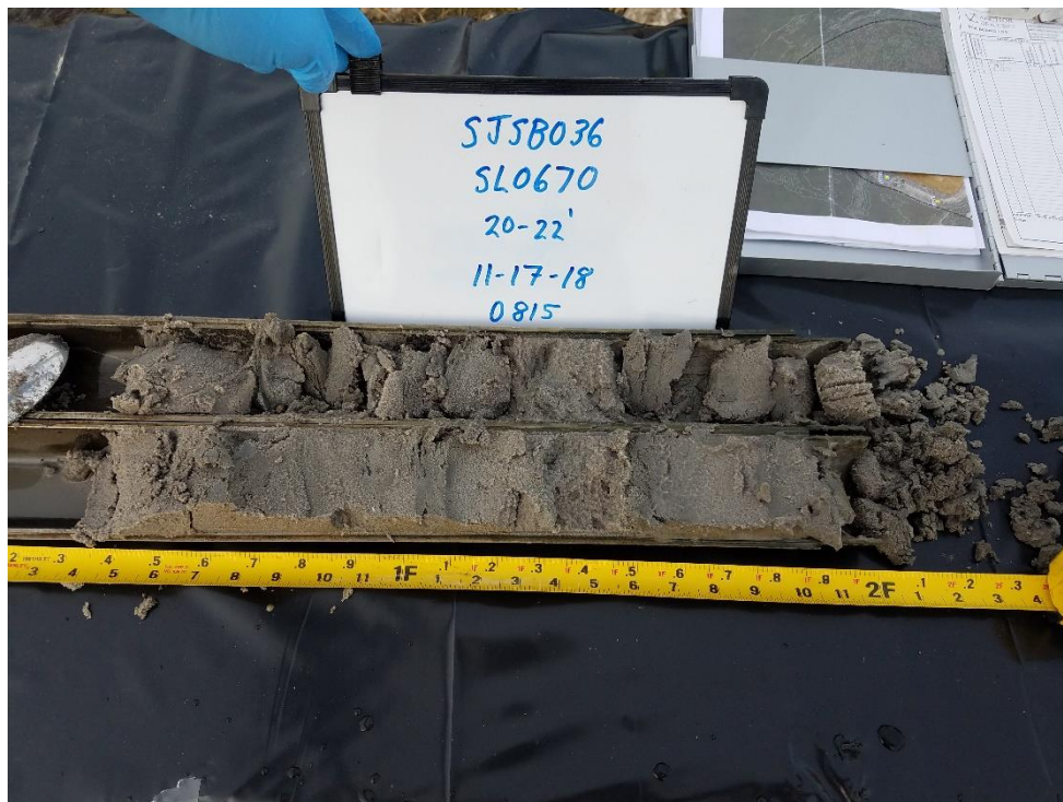
Photo 47 - Geotechnical Sample SJSB036 (20-22)
