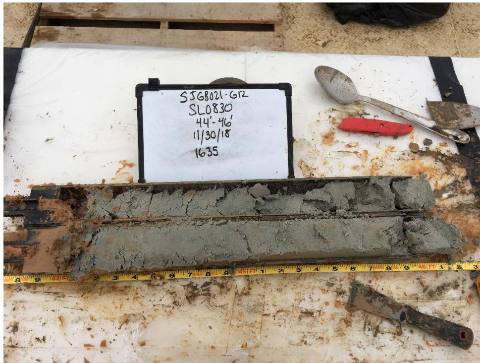
Photo 8 - Geotechnical Sample SJSB021 (44-46)
