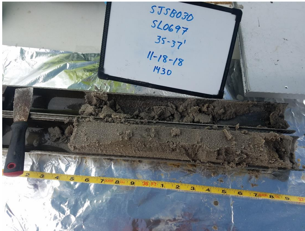
Photo 24 - Geotechnical Sample SJSB030 (35-37)
