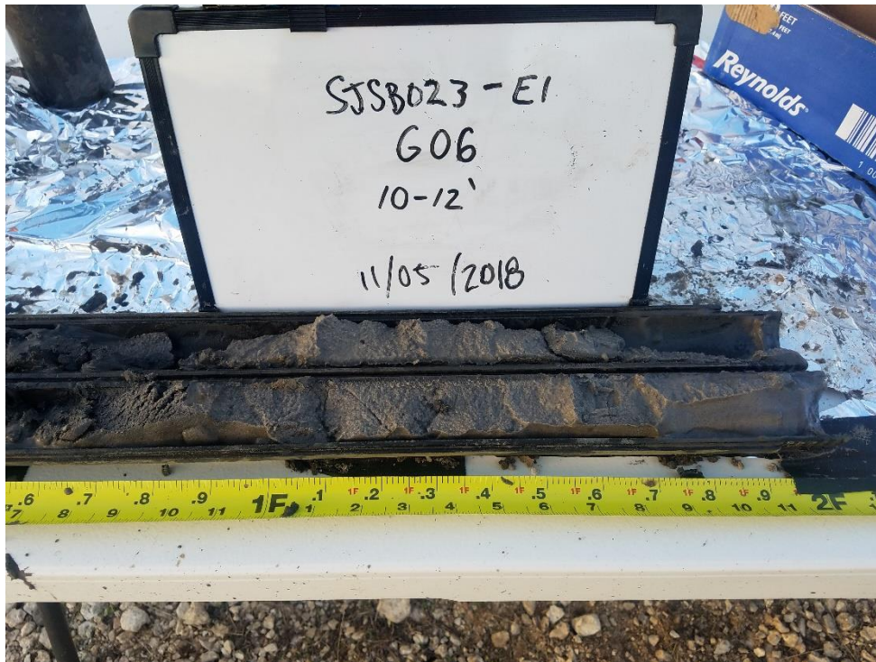
Photo 40 - Geotechnical sample from location SJSB023-E1 at 10 to 12 ft.
