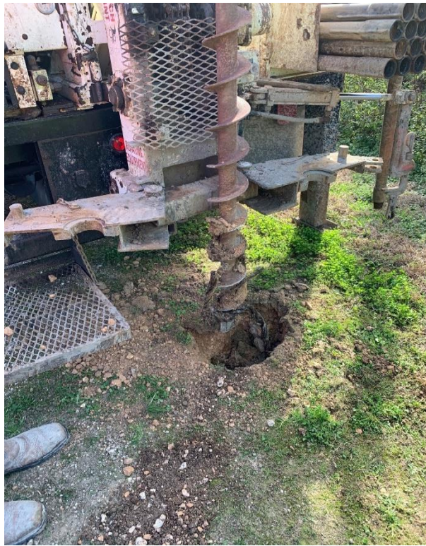
Photo 5 - Debris wrapped around hollow stem auger at location SJGB028.
