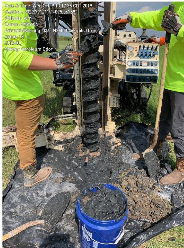
Photo 4 - Drill crew collecting treatability study samples using hollow stem augers.
