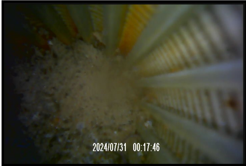
PS11 – sand bottom after only a couple of feet
