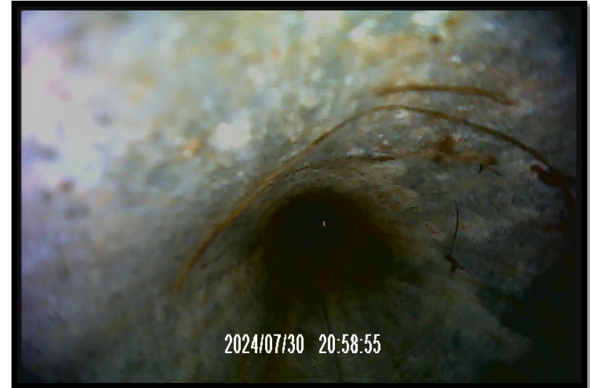
COP1 – minor indentation in casing
