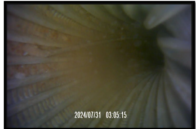
PS4 – bend in screen and build up along left side
