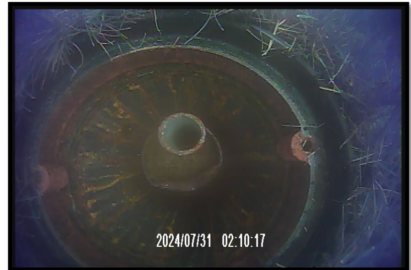
PS6 – well within flush mount, no cap when opened
