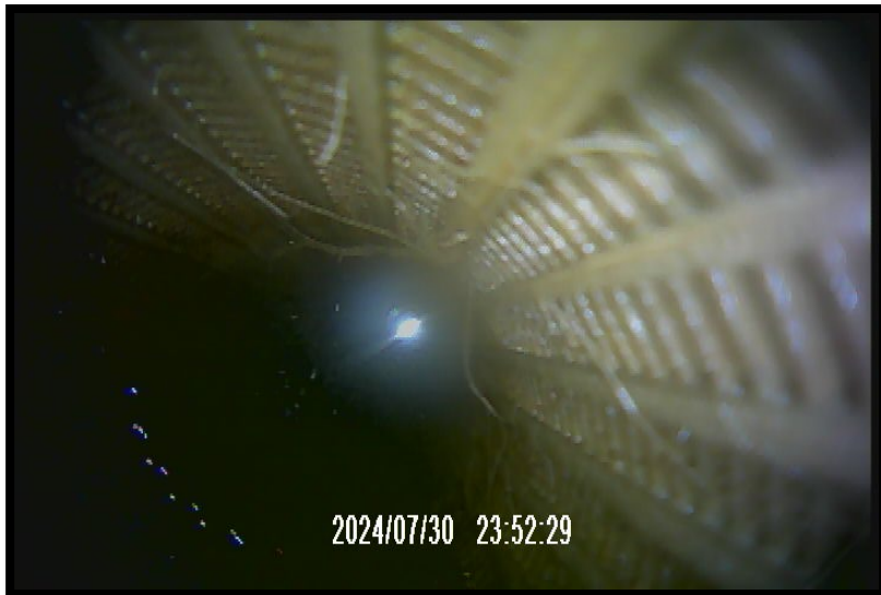
COP3 – possible roots getting into screen, water table reflection
