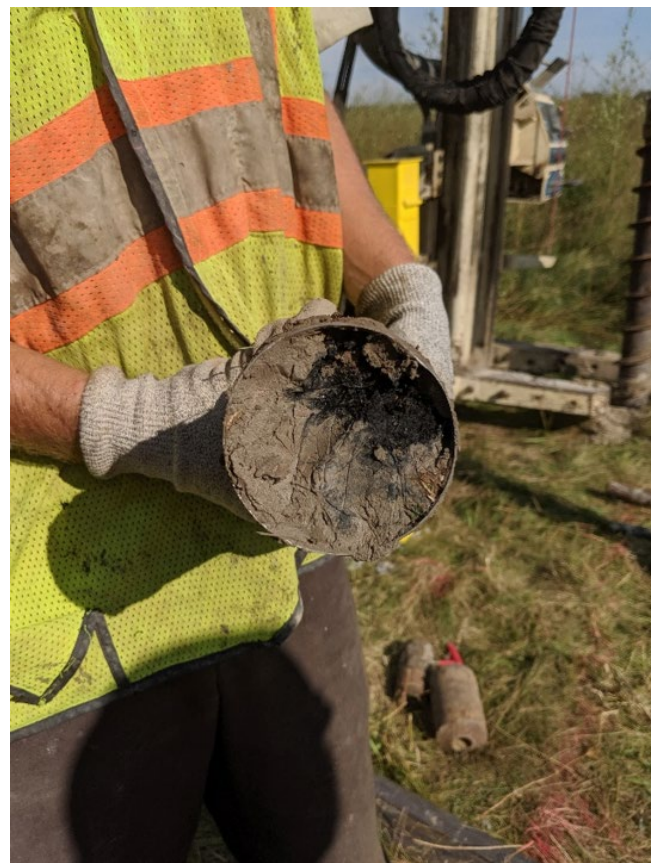
Collection of slurry wall material sample.
