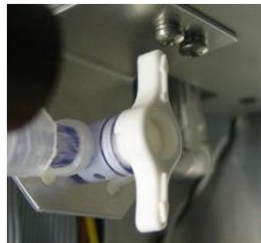
Purge valve closed (Left) and open (Right). Located inside the battery compartment
