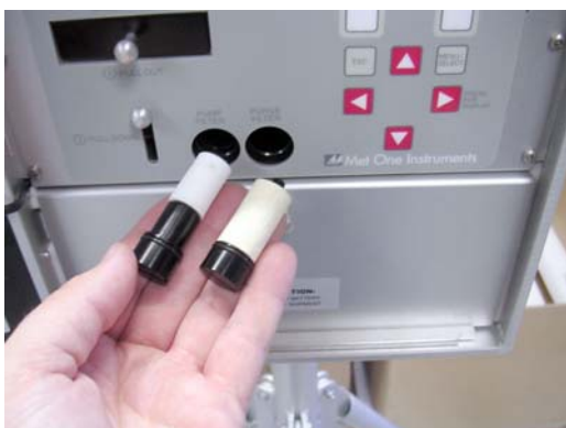
Pump Filter and Purge Filter Replacement
