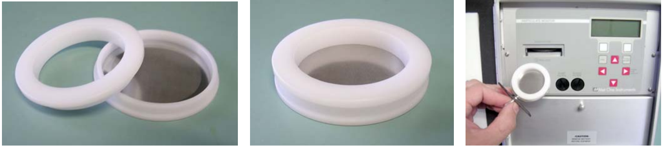
The 47 mm Filter Cassette and Filter Tray
