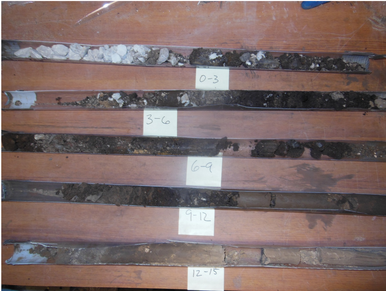
Existing soil conditions at on-track locations
